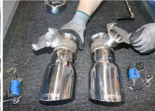
10. Confirm the spring wire form is correctly positioned on the passenger side stock valve actuator from Removal Step 7. Position and install passenger valve actuator onto the CORSA passenger valve tip assembly. Confirm that the spring wire form is located within the grooves of the valve assembly.
