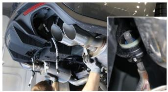
5. Slide the stock exhaust assembly rearward until the stock resonator and sleeve clamps are free from the exhaust manifold pipes. Lower the front of the exhaust then slide it forwards to remove the rear driver and passenger side hangers from their hanger grommets and remove the exhaust from the vehicle.
