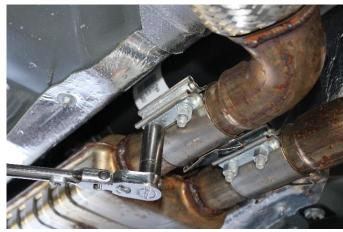
2. Slide the stock tunnel muffler inlet pipes into the sleeve clamps. Center the tunnel sections within the vehicle tunnel cavity and snug the clamps using a 15mm deep socket and 3/8" drive ratchet. Place a jack stand or similar device under the stock tunnel muffler for support.
