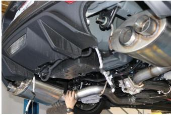
**8.** Repeat **Install Steps 4-7** on the driver side of the vehicle. Once the system is secure, it is safe to remove the jack stand from beneath the X-Pipe.
