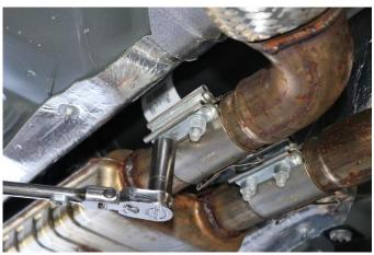
**3.** Use a flat head screw driver to pry open the locking spring tab on both of the sleeve clamps at the cat-back connection point.
