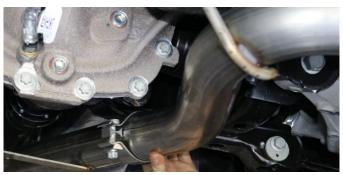
**5.** Slide the rear hanger into the passenger rear hanger grommet located just inside the passenger side tip cut out. Slide the muffler inlet pipe over the passenger side X-Pipe outlet.
