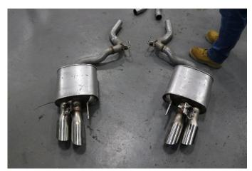
**14.** Use a chain cutter or similar device to cut both the driver and passenger side exhaust pipes at the marked locations.
