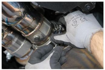
14. Mate the v-band flange on the driver valve tip assembly to the flange on the muffler. Align and position the v-band flange so both flanges are fitted within the grooves of the clamp. Reinstall the lock nut and snug the clamp using an 11mm deep socket and 3/8" drive ratchet. The clamp should be positioned with the lock nut towards the inside of the vehicle, the bolt on top and horizontal.
