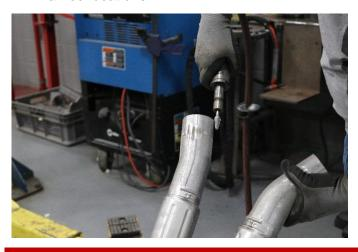
**15.** Use a file or similar device to file any burrs on the cut end of the stock tunnel section on both outside and inside edges. Place the stock tunnel section in a safe location for **Install Step 2**.
