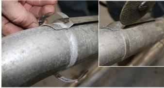
10. Using a cut off wheel or similar device, carefully cut the band clamp holding the rear most heat shields. Use caution as to not cut into the exhaust pipe itself.
