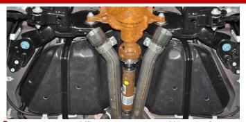
3. Install two, 2 ½" clamps on the 2 ½" end of the CORSA Axle-Back adapters so the bolt is vertical and towards the inside of the vehicle, with the nut towards the ground. Slide adapters over factory tunnel muffler outlet pipes, and tighten clamps using a ratchet and 15mm deep socket, until adapters are snug on the pipes.
