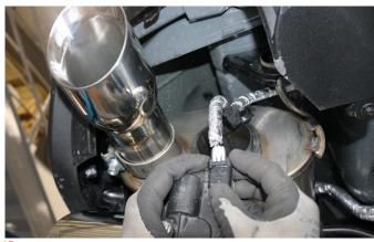
13. Connect the driver side harness into the actuator mounted to the driver valve tip assembly by pushing the plug until you hear a click, followed by the white locking clip.
