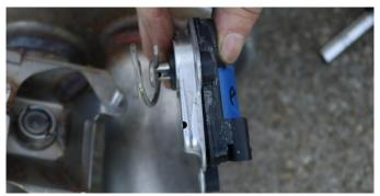
7. Use a 3/8" drive ratchet and a 10mm socket to remove the three nuts on each actuator. Remove the actuators from their valve assemblies. Place the actuators in a safe location to be used during Install Step 10. Install the hardware back onto the studs or store in a safe location since they will not be re-used during installation.
