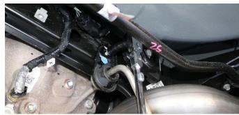
6. Install the front passenger hanger grommet assembly onto the rear suspension sub-frame and tighten down with the 13mm bolt from Removal Step 4, using a 3/8" ratchet and 13mm socket.
