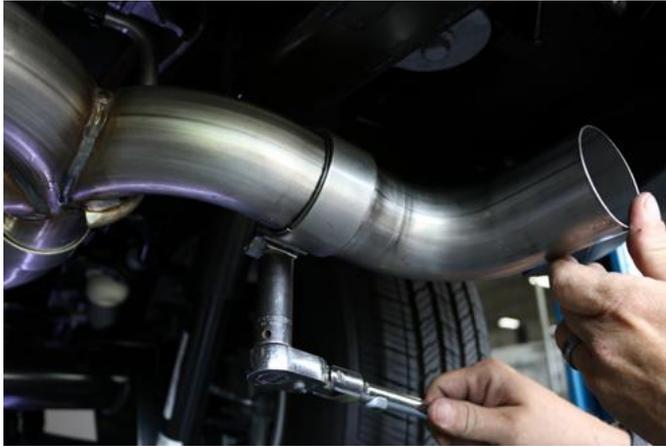
7. Place a clamp on the expanded end of the 90-degree elbows with the hardware toward the front of the vehicle with the nut down. Then slide that end over the outlet pipe of the muffler. Use a 15mm socket or wrench to snug the clamp. Repeat for the other side.
