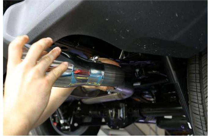
8. Slide the tips onto the tip elbow pipes with the etch centered on the top of each tip. Snug the bolt on the clamp using a 13mm socket or wrench.
