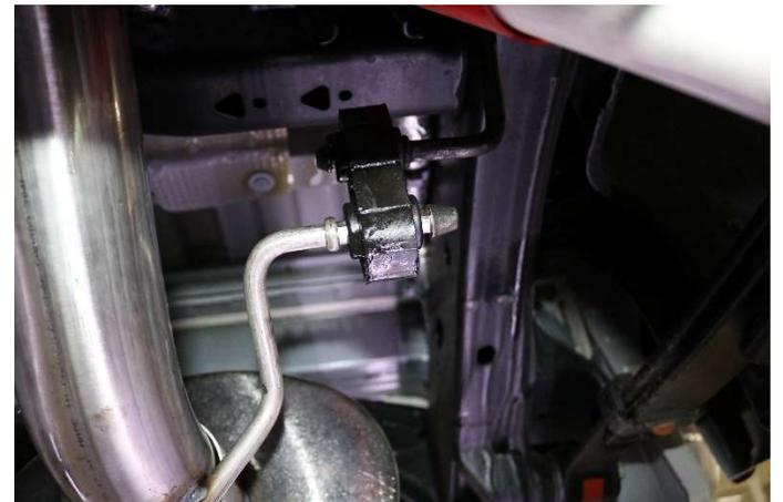
**10.** Insert the front hanger on the Passenger side of the Tailpipe Assembly into the factory hanger grommet as shown.
