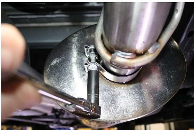
**13.** Snug the 3" TORCA clamp next to the muffler on the tailpipe using a 15mm socket.
