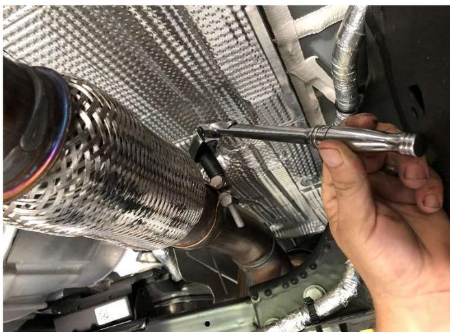
3. Use a 13mm socket to loosen the spherical clamp on the factory headpipe. Keep the factory spherical clamp for use with your Corsa Exhaust System.
