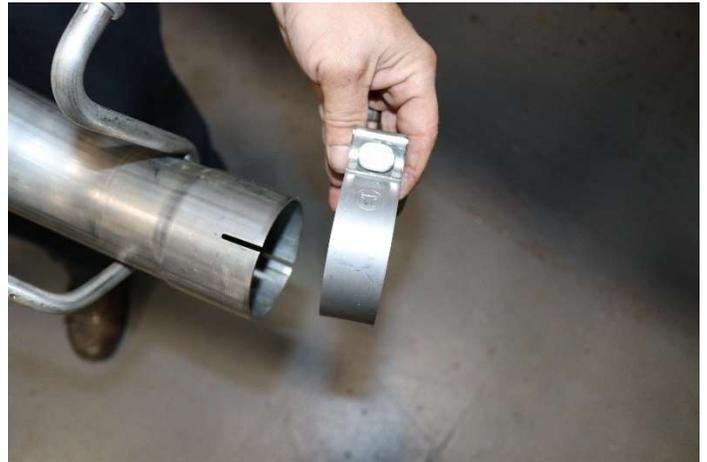
**8.** Insert a 3" TORCA clamp into the expanded and notched end of the TailPipe Assembly as shown.
