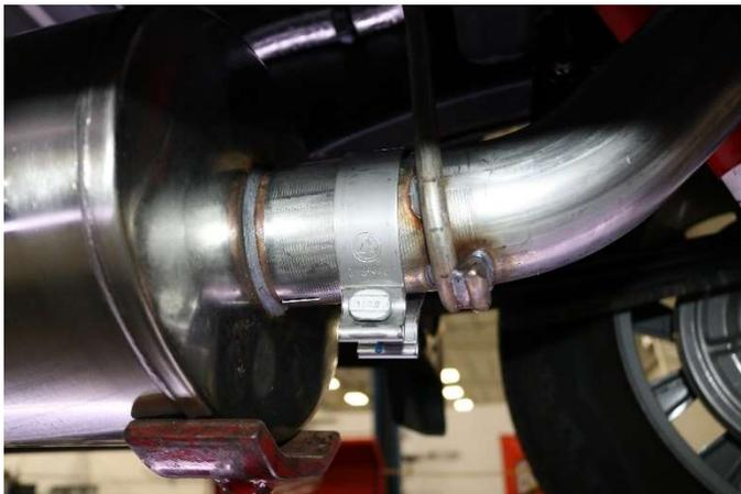
**9.** Slide the TailPipe Assembly into the side of the muffler supported by the stand as shown.
