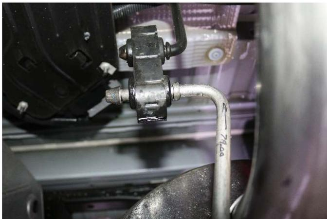
**11.** Insert the front hanger on the Driver's side of the Tailpipe Assembly into the factory hanger grommet as shown.
