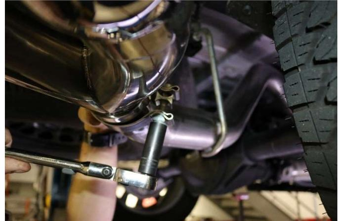
**16.** Snug the TORCA 3" Clamp on the tip assembly using a 15mm socket.
