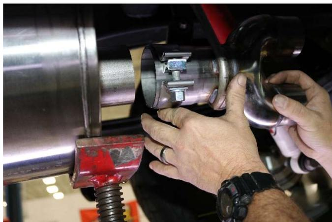
**10.** Slide the Y- Pipe Assembly into the side of the muffler supported by the stand as shown.
