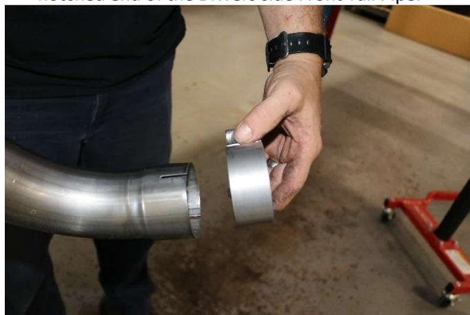
**15.** Insert a TORCA 2.5" Clamp into the expanded and notched end of the Passenger side Front Tail Pipe.
