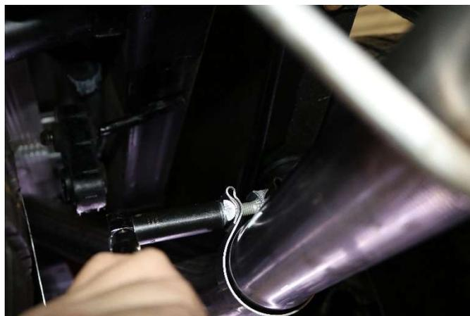
**22.** Visually inspect the exhaust system position, alignment, clamp orientation & position and exhaust system clearances. Make any adjustment necessary at the slip joints.
