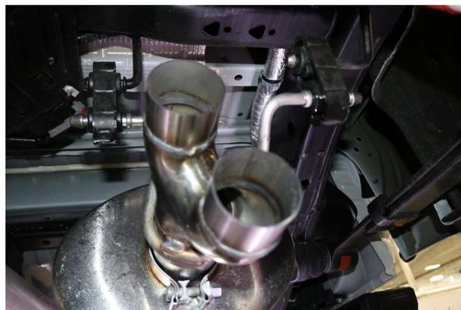
**11.** Insert the hangers on the Y-Pipe Assembly into the factory hanger grommets as shown.
