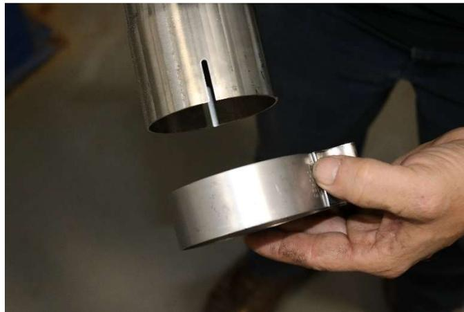
**9.** Insert a 3" TORCA clamp into the expanded and notched end of the Y – Pipe Assembly as shown.
