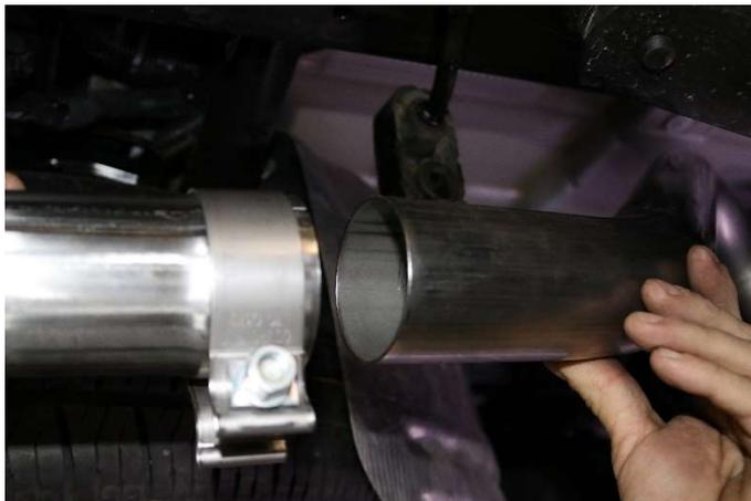
**20.** Slide the expanded and notched end of the passenger side rear tailpipe into the passenger side front tailpipe. Snug the TORCA 2.5" clamp using a 15mm socket.
