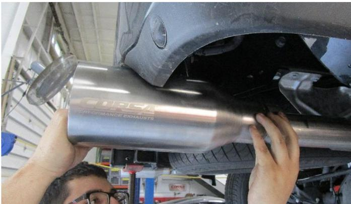
**11.** Place a 2.5" clamp into the inlet of the tips and Install tips on to both driver and passenger side of the vehicle. Adjust length and rotation to get the corsa etch on to the side of tips and to get the tip dept even between driver's and passenger side.
