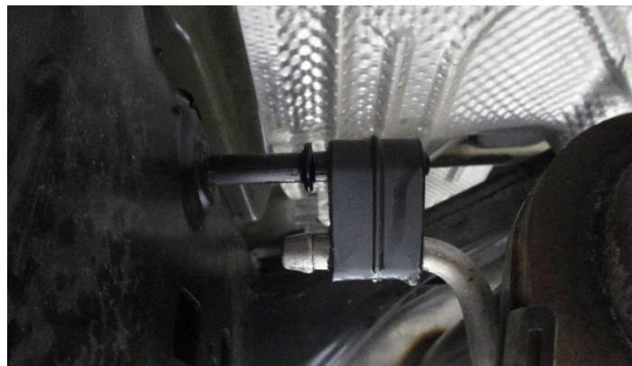
**4.** Place the front muffer hanger in the factory grommet.
