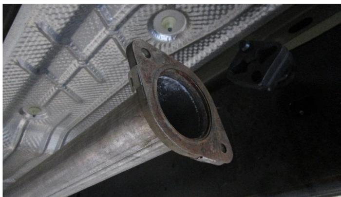
**1.** Place the gasket that was taken off from the factory exhaust system and place on the mid pipe flange.
