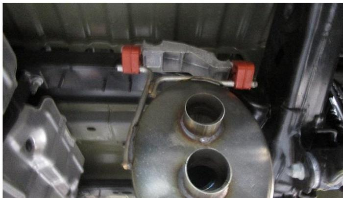
**3.** Place rear muffer hangers in the factory grommets.
