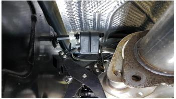
**6.** Remove the hanger from the front of the muffler using a Grommet puller or similar device.
