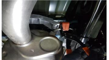
Remove both of the hangers from the grommets at the back of the muffler using a Grommet Puller or Similar Device.
