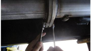
Using a 17mm socket or wrench for the bolt, and a 15mm socket or wrench for the nut, secure the flange connection with the supplied hardware.
