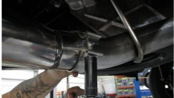
**12.** Using a 15mm socket or a wrench, snug the tip clamp to leave room for adjustment.
