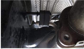
**3.** Place the front muffler hanger in the factory grommet.
