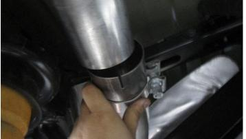
8. Install a 3" clamp to the inlet of the rear tailpipe as shown then insert the rear tailpipe on the outlet of the front tailpipe as shown.
