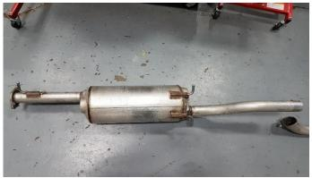
**1.** Carefully guide the factory muffler and the front tailpipe assembly towards the front of the vehicle and down to remove the system completely from the vehicle.
