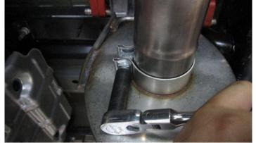
**1.** Secure the clamp using a 15mm socket or a wrench. **DO NOT** fully tighten at this time.
