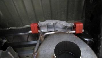
**4.** Place the rear muffler hangers in the factory grommets.
