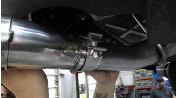
Place a 3" clamp into the inlet of the tip and install the tip into the rear tailpipe. Adjust the length and rotation of the tips per your preference.
