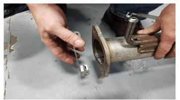
8. Remove the factory gasket from the muffler and save it to reuse it for the Corsa System.
