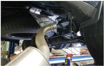
**3.** Carefully remove the rear tailpipe from the vehicle and place it aside.
