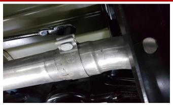
**1.** Loosen rear tailpipe clamp using a 15mm socket or wrench.
