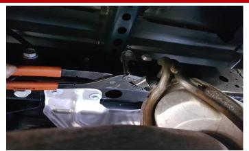
2. Remove rear tailpipe hanger using a Grommet Puller or Similar Device.
