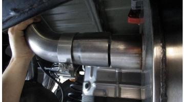
**6.** Install a 3" clamp to the inlet of the front tailpipe as shown then insert the front tailpipe on the outlet of the muffler as shown.
