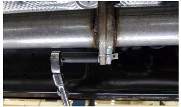
**4.** Loosen and remove the two muffler flange bolts that secure the muffler inlet flange using a 16mm socket or a wrench.
