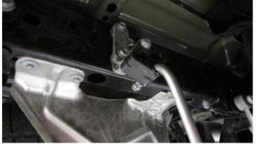
**10.** Insert the rear tailpipe hanger into the factory grommet.
