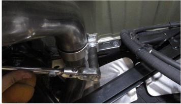
**9.** Secure the clamp using a 15mm socket or a wrench. **DO NOT** fully tighten at this time.
