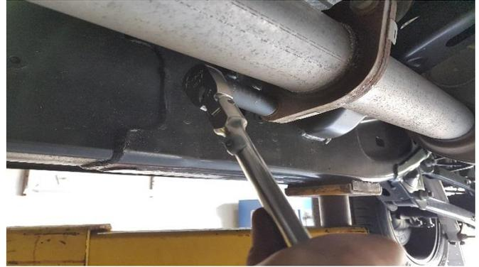
**2.** Remove the bolts from the rear flange using a 16mm socket or wrench.
