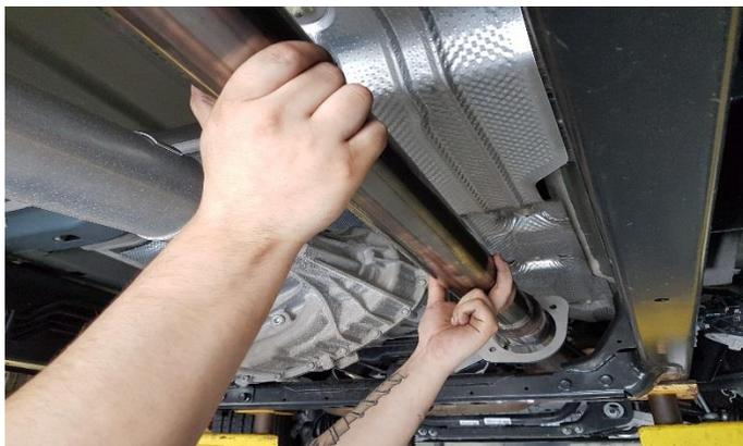
**1.** Install Corsa Res Delete assembly as shown.
