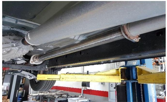
4. Center the flare, and the floating flange and tighten the nuts on the floating flange to 40FT/LBS and then tighten the nuts on the rear flange to 35 FT/LBS.
