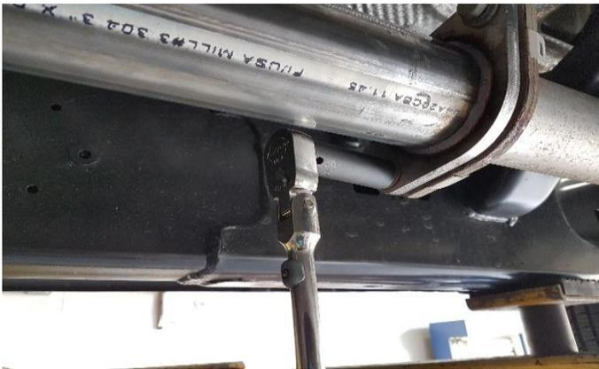
3. Align the rear flange with the mating flange on the muffler. Position the stock 16mm bolt on the rear flange and snug it using a 16mm socket or wrench.
