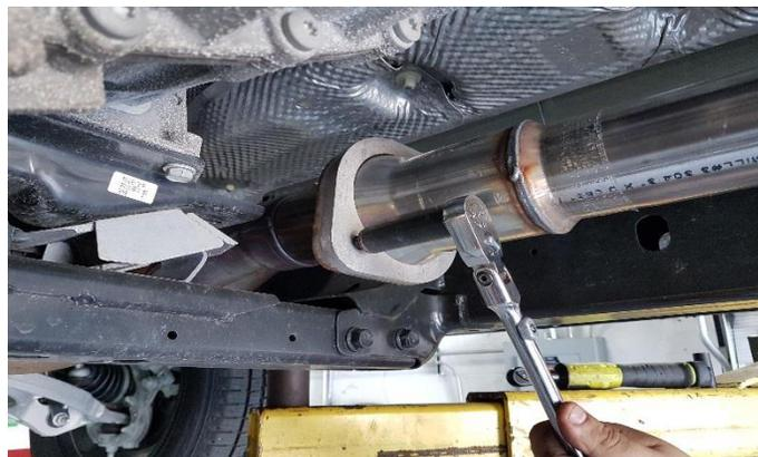
**2.** Position the floating flange and secure the stock 15mm nuts on the bolts using a 15mm socket and ratchet. Only Snugly tighten at this time.
