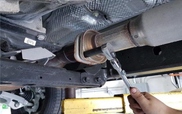
**1.** Remove the nuts from the front flange using a 15mm socket or wrench.
