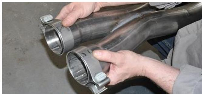
**2.** Install two 3" clamps on the driver and passenger inlets of the Double X-Pipe so that the bolts are vertical with the nut towards the ground and the bolts towards the outside of the vehicle.
