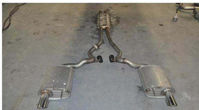
4. Slide the stock exhaust assembly rearward until the stock resonator inlet pipes are free of the sleeve clamps. Lower the front of the exhaust in order to create clearance between the resonator inlet pipes and the sleeve clamps. Slide the complete exhaust forwards to remove the rear driver and passenger side hangers from their respective hanger grommets and free the stock exhaust from the vehicle. **NOTE:** The use of a soap and water solution may aid in the removal of hanger grommets.
