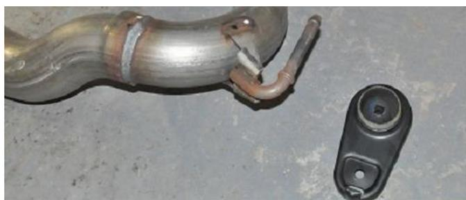
5. Remove the driver and passenger side hanger grommet assemblies from the front muffler hangers using grommet pullers or a similar device. **Save for reinstallation (Install Step 5).** **NOTE:** The use of a soap and water solution may aid in the removal of hanger grommets.
