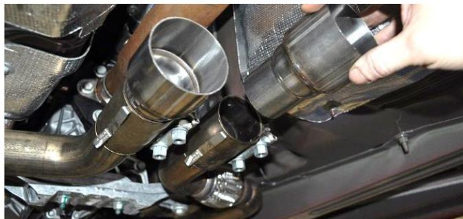
**1.** Locate the two X-Pipe inlet adapters. Slide the adapters into the factory sleeve clamps, and tighten using the ratchet and 15mm deep socket, until the adapters are snug in the clamps.
