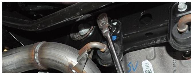
2. Use a 3/8" drive ratchet and 13mm socket, to remove the bolt holding down the driver side hanger grommet assembly.
