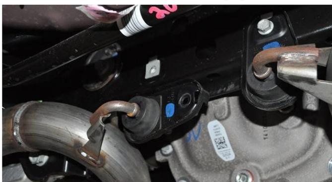
3. Once the bolt is removed, push up slightly on the exhaust and slide the hanger grommet assembly rearward to free it from the rear suspension sub-frame. Rotate the hanger grommet assembly a minimum of 90° so that it will not interfere with the rear suspension sub-frame. **Save bolt for reinstallation (Install Step 9).** Repeat on the passenger side hanger grommet assembly.
