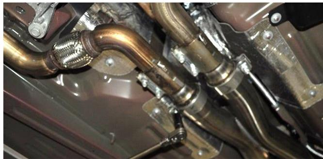
**4.** Position the X-Pipe so the cross brace located at the rear of the X-Pipe is facing down and parallel with the ground, and the outlets are centered around the differential. Tighten the clamps using a ratchet and 15mm deep socket, until the X-Pipe is snug on the adapters. Place a jack stand or similar device under the X-Pipe for support.
