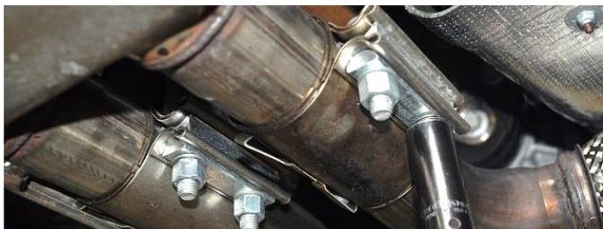
1. Use a 3/8" drive ratchet and 15mm deep socket, to loosen the two sleeve clamps at the cat-back connection point. Both nuts must be loosened in order for the clamp to fully disengage.
