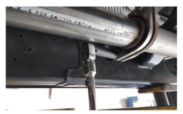
Align the rear flange with the mating flange on the muffler. Position the stock 16mm bolt on the rear flange and snug it using a16mm socket or wrench.
