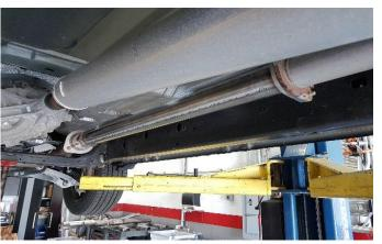
4. Center the flare, and the floating flange and tighten the nuts on the floating flange to 40FT/LBS and then tighten the nuts on the rear flange to 35 FT/LBS.
