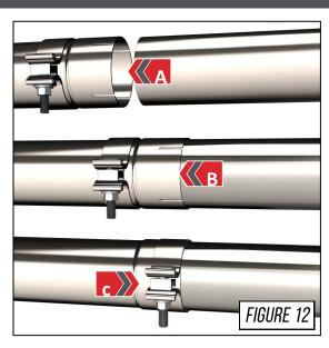
To accomplish the best tip fitment, align the 2.5" tip clamp to cover *only* the slot, as shown by **Arrow A** in **Figure 13**.
