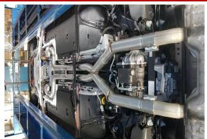
15. Now adjust the entire exhaust system. Ensure the adapter overlaps, the rear tip depth and rotation so that the tips are centered and aligned. Check the position of all hangers to make sure they are properly seated within their corresponding grommets. Check clearances between the system components and chassis.
