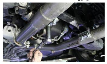
14. Snug the Clamp Nuts with a 15mm socket (or wrench), but do not tighten, it may hinder proper alignment of the entire system. These will be torqued later in the installation. Ensure the Clamp Nut and Stud are vertical while snugging.
