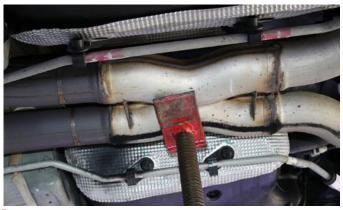
Support the Factory Crossover Pipe using a jack stand or similar device.
