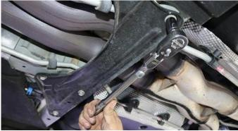
17. Then reinstall the Cross Member with a 13mm socket (or wrench) and the 5 Factory bolts. Tighten all bolts to the manufacturer's specifications.
