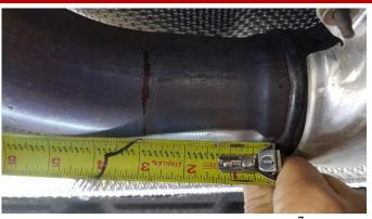
**6.** Starting on the Driver-side, measure  $2\frac{7}{8}$ " from the underside of where the Pipe welds to the factory secondary catalytic convertor, following along the underside profile of the Factory exhaust pipe. The tape measure must follow the bend profile of the pipe. Mark the pipe at the measured point to create a cut line.
