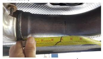
7. On the Passenger-side, measure  $4\frac{1}{8}$ " from the underside of where the Pipe welds to the factory secondary catalytic convertor, following along the underside profile of the Factory exhaust pipe. The tape measure must follow the bend profile of the pipe. Mark the pipe at the measured point to create a cut line.
