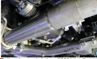
13. Note: If you are installing a CORSA Axle Back kit, complete its installation before continuing. When the CORSA Axle Back kit is installed, resume this installation. Slide the Sleeve Clamps over the compressed end of the Rear Adapters.
