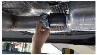
**3.** Locate new Driver-side Head Pipe and slide it into the factory cut pipe with the clamp as shown.
