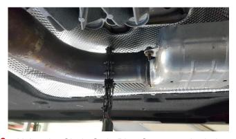
**8.** Using the Chain Style Pipe Cutter, cut both the Driver and Passenger Factory Exhaust pipes at the marked locations.
