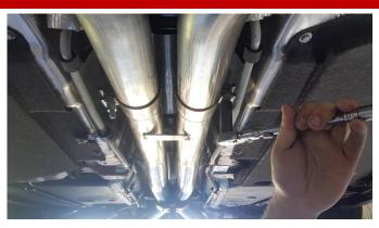
Snug the Clamp Nuts with a 15mm socket (or wrench), but do not tighten. Tightening now may hinder proper alignment of the entire system. These will be torqued later in the installation. Ensure the Clamp Nut and Stud are vertical while snugging
