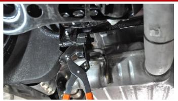
5. Note: If you are installing a CORSA Axle Back kit, skip this step and refer to Steps 3 and 4 in the Removal section of the CORSA Axle Back instructions. Remove the two Hangers on the rear each side from the Factory Grommets using the Exhaust Hanger Removal Pliers or a similar device. Note: Careful not to damage the Grommets during removal. (Will be reused during installation)
