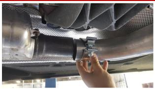
1. Locate new Passenger-side Head Pipe and slide it into the factory cut pipe with the clamp as shown.
