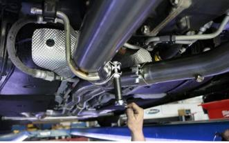
12. Snug the Clamp Nuts with a 15mm socket (or wrench), but do not tighten. Tightening now may hinder proper alignment of the entire system. These will be torqued later. Ensure the Clamp Nut and Stud are vertical while snugging.
