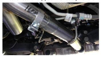
**10.** Next, rotate the Rear Adapter Pipe and slide the flared end of the Rear Adapter over the rear leg of the Single X-pipe. Do <u>not</u> slide the Sleeve Clamps on at this time.
