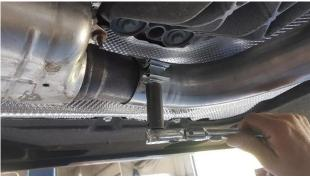
Snug the passenger side head pipe clamp to allow for minimal movement enough for adjustment.
