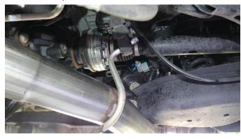
**8.** Locate the Driver-side Rear Adapter Pipe. Apply the soap and water mixture onto the Hanger Rod and into the hole in the Grommet. This will help them slide and ease Hanger installation. With the flared end of the Rear Adapter Pipe towards the engine, insert the Hanger Rod into the hole in the Grommet.
