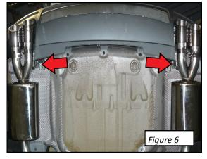
Once tips are centered and level, tighten the cross-bracket and rubber hanger mount fasteners.
