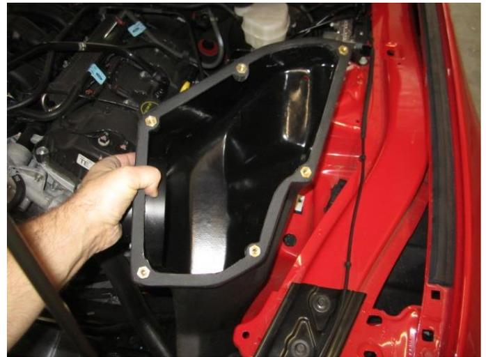
8. Place the CORSA air box into the factory location the air box will slide over the factory inlet.
