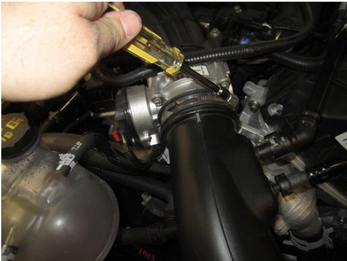
3. Loosen the clamp holding the duct to the throttle body.
