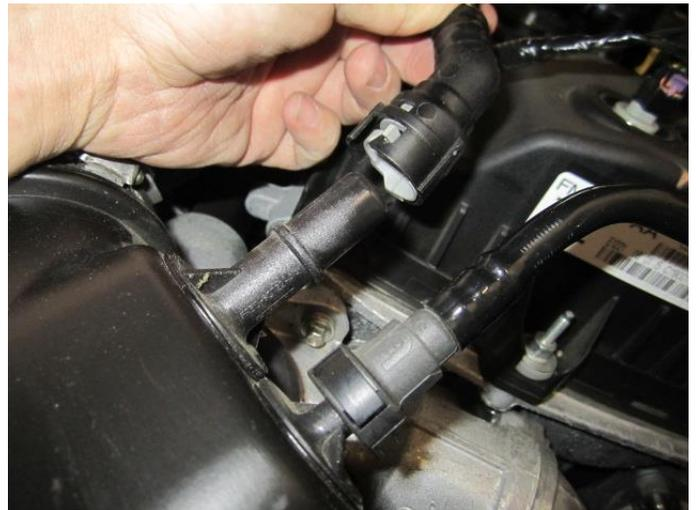
4. Disconnect the factory breather hoses from the factory air duct.
