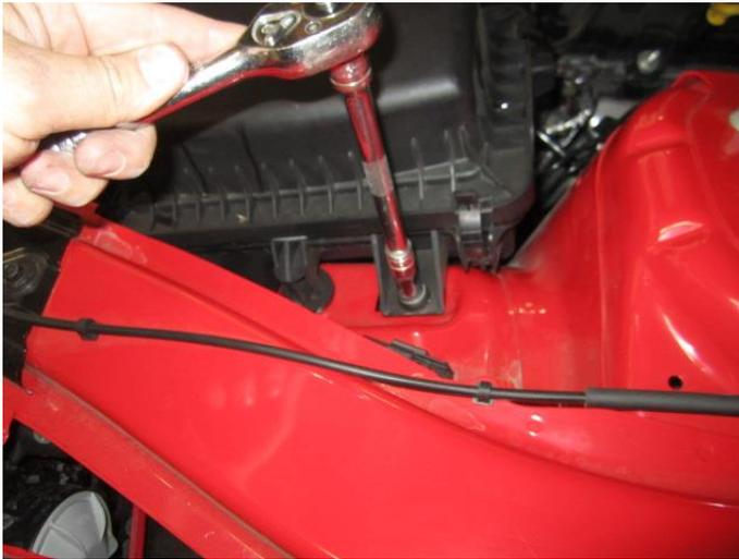
1. Remove the 10mm bolt holding the factory air box in place.
