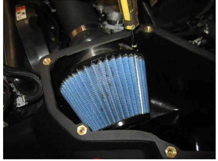
18. Tighten the #5120 Pro-5 filter onto the adapter using a 5/16 socket or nut driver only.
