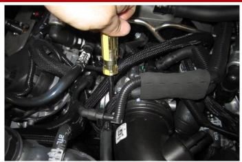
**1.** Loosen the clamp holding the factory air duct to the throttle body.
