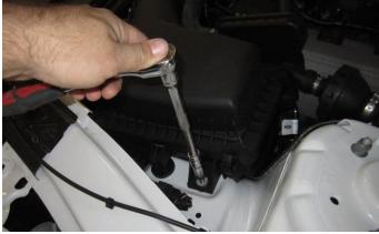
Remove the 10mm bolt holding the factory air box in place. Save bolt for reinstallation (Install Step 2).
