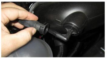
Disconnect the idle hose from the factory air duct
