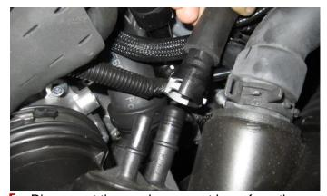
Disconnect the crankcase vent hose from the factory air duct.
