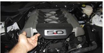
1. Remove the engine cover by lifting up and out. Save for reinstallation (Install Step 15).
