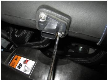
Attach the factory MAF sensor onto the CORSA air duct with the provided MAF gasket and 4mm screws.
