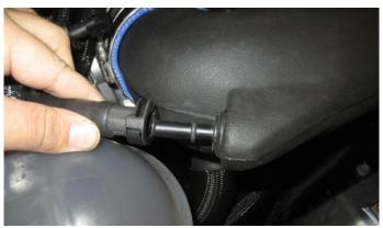
11. Attach the idle bypass hose onto the 3/8 snap fitting on the CORSA air duct
