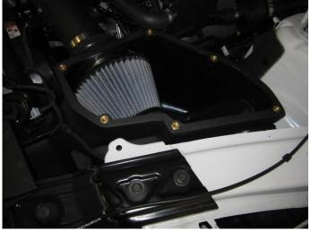
**16.** Attach the #5120 filter onto the filter adapter and tighten into place using a 5/16 socket or nut driver only.
