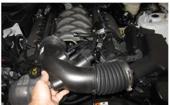
Remove the factory air duct from the engine compartment.
