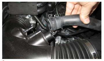
Disconnect the sound tube from the factory air duct.
