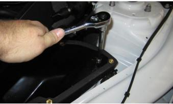
2. Tighten the air box in place using the factory 10mm bolt from **Removal Step 10**.
