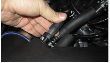
**12.** Attach the EVAP, crankcase vent line and sound tube onto the CORSA air duct.
