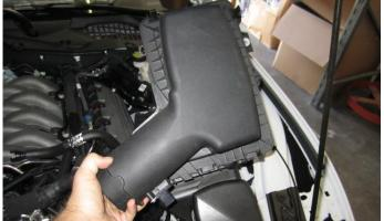
12. Remove the factory air box from the engine compartment then remove the tree rivet holding the MAF sensor harness onto the wheel well.
