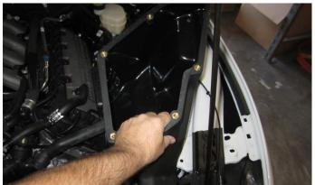
Slide the CORSA air box over the factory air inlet. PRO TIP: The use of a flathead screwdriver may aid in sliding the CORSA intake over the stock inlet.
