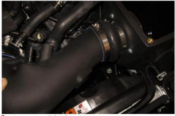
**1.** Press the CORSA air duct into the 4in hump hose, do not tighten the clamp at this time.
