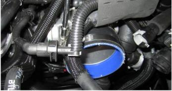
**6.** Attach the 3.5 x 2.5 sleeve onto the throttle body with a #56 clamp using a 5/16 socket or nut driver only.
