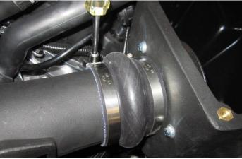
Tighten the CORSA air duct onto the hump hose with a #64 clamp using a 5/16 socket or nut driver only.
