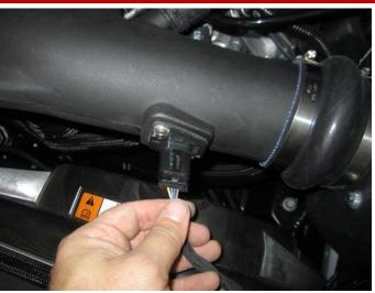
**14.** Attach the MAF sensor harness onto the MAF sensor.
