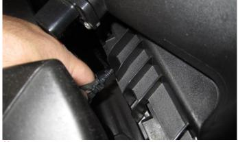
**11.** Remove the tree rivet holding the MAF sensor harness to the factory air box.
