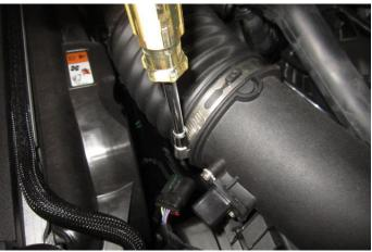
**8.** Loosen the clamp holding the factory air duct to the air box.
