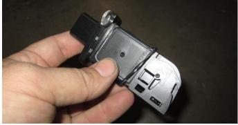
**5.** Remove the O-ring from the MAF sensor. **Save for reinstallation** (Install Step 13)
