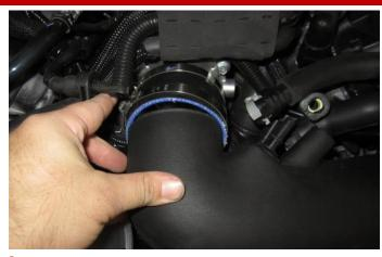
**8.** Press the CORSA air duct into the 3.5in sleeve.
