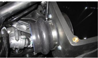
Attach the 4in hump hose onto the filter adapter with a #64 clamp using a 5/16 socket or nut driver only.
