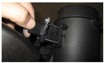
**4.** Carefully remove the factory MAF sensor from the stock air box.
