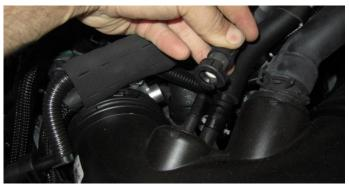
Disconnect the EVAP hose from the factory air duct
