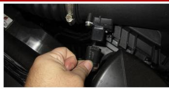
**2.** Disconnect the MAF sensor harness from the MAF sensor.
