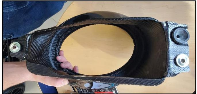
2. Assemble the 3 stock Mount Hardware into the CORSA Carbon Fiber Air Box in the same orientation and position as stock.
