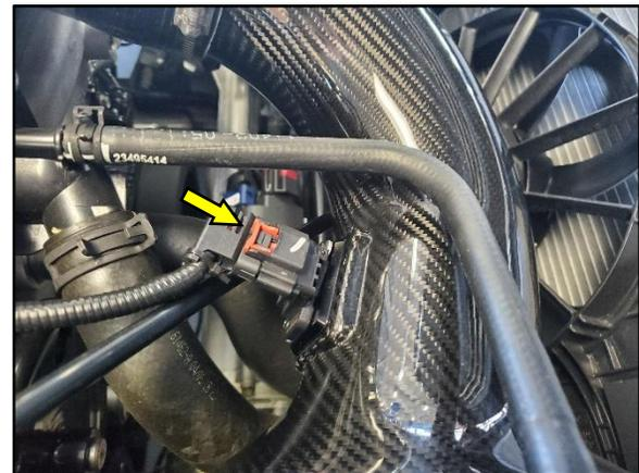
**13.** Locate the MAF Sensor Harness and push Plug onto the MAF Sensor. Push the **RED** Clip down on MAF Sensor Plug to lock it in place.
