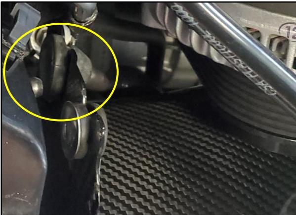
3. Install the CORSA Carbon Fiber Air Box by first pushing the Lower Rear Mount onto the Stud on the Fender
