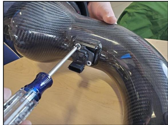
8. Locate the stock Air Box, then locate and remove the 2 MAF Screws. The screws will NOT be reused.
