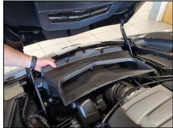
1. Locate and remove the 4 Screws securing the Radiator Air Outlet Duct with a 7mm Socket & Ratchet or Nut Driver.
