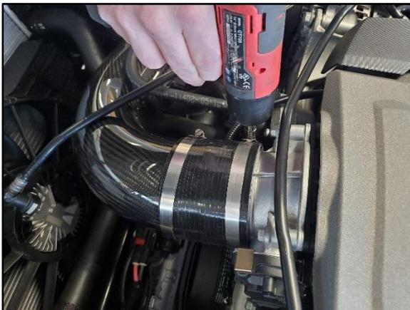
**12.** Insert the Silicone Sleeve onto the CORSA Carbon Fiber Air Duct, then slide the 2 Clamps over the Silicon Sleeve. Next, insert the Silicon Sleeve onto the Throttle Body. Using an 8mm Socket & Ratchet or Nut Driver, torque the Hose Clamps to 44 in-lbs (5 N-m).
