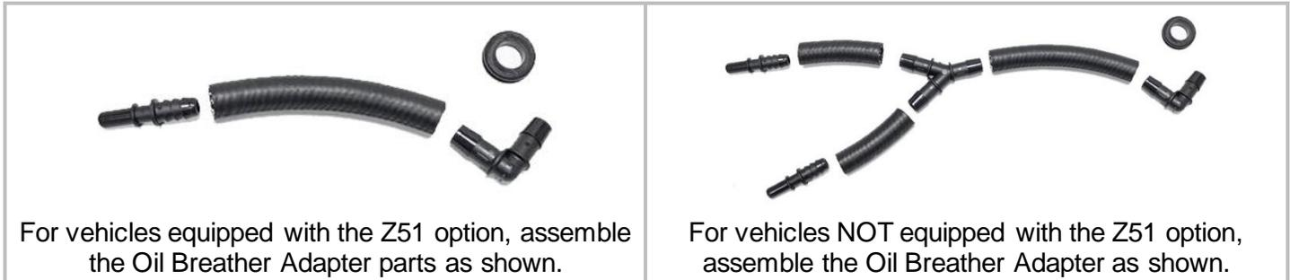
5. Fully insert the Fittings into the Hose(s). If the 652117 –  $\text{Ø}1/2$ ” to  $\text{Ø}3/8$ ” Bundy Fittings (Part #11 above) feel loose, use the included clamp to secure them in the hose.
