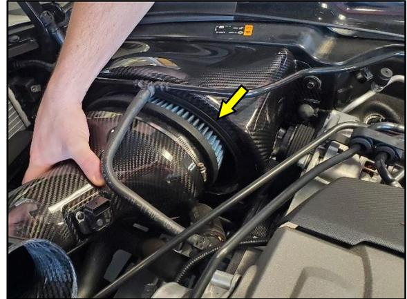
**11.** After ensuring the Gasket is in place on the CORSA Carbon Fiber Air Box opening, carefully insert the CORSA Carbon Fiber Air Duct and Filter into the Air Box. Double check the Gasket between the Air Box and Air Duct is not pushed into the Air Box. When fully installed, the Filter and Clamp will not be visible.
