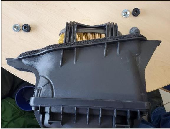
1. Note the orientation and position of the 3 stock Mount Hardware and then carefully remove them from the stock Air Box. These will be reused.
