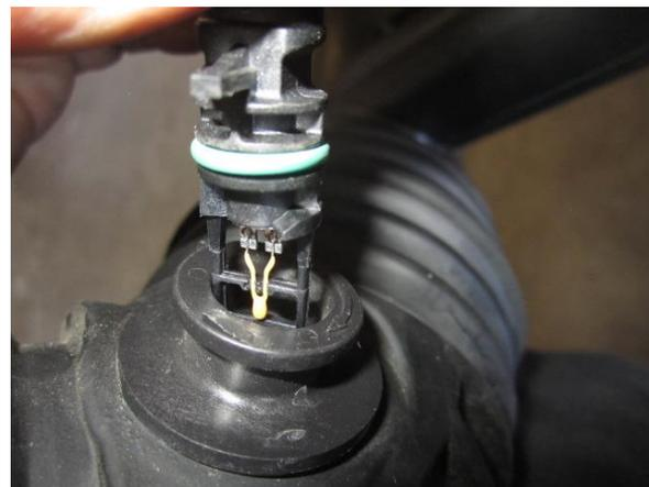
4. Locate the factory air duct and remove the air temperature sensor by gently lifting tab and twisting counterclockwise then pulling straight out.
