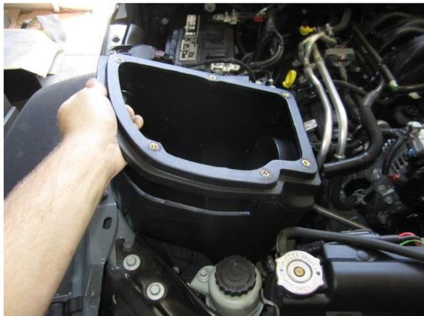
1. Locate CORSA air box and place into factory position in vehicle.
