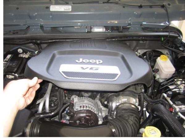
2. Remove engine cover by pulling up on the front then pulling cover out.
