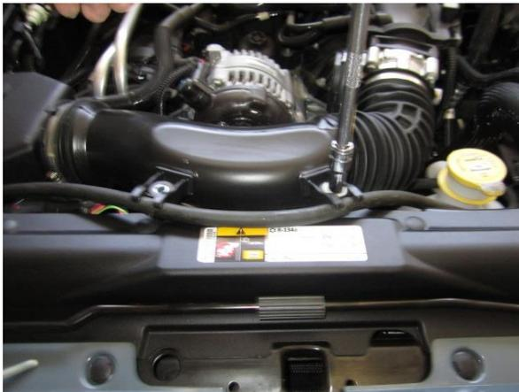
3. Remove the two bolts securing the factory air duct to the core support using a ratchet and 10mm socket.
