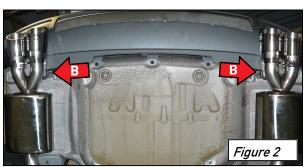
Once tips are centered and level, tighten the cross-brace and rubber hanger mount fasteners.
