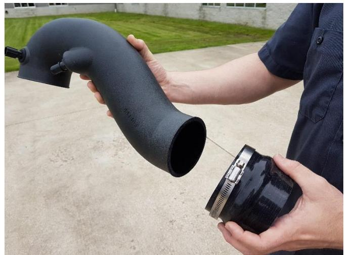
**13.** Install a 4" Clamp onto one end of the hump hose and slide it onto the duct.
