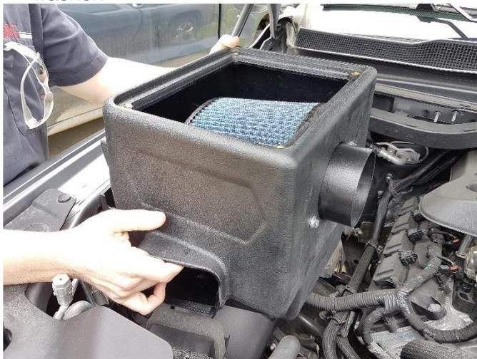
**8.** Align the four grommets in the Corsair box to the four mounting points in the car as shown.
