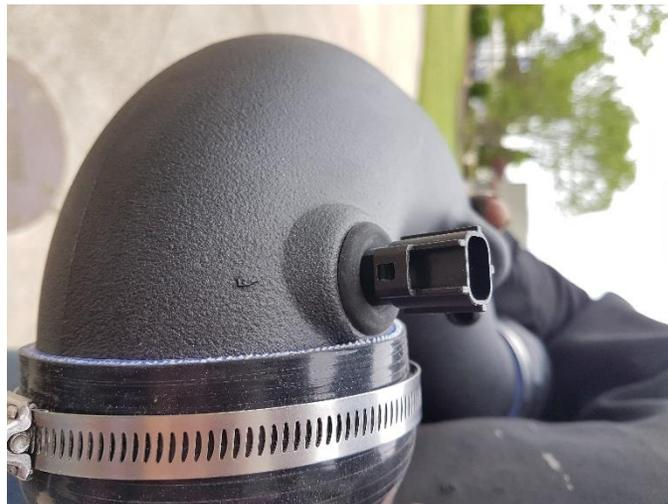
**2.** Turn the sensor such that the sensor clip for the harness is facing the arrow in the duct.
