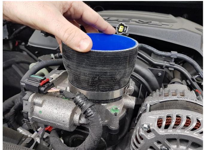
**11.** Install the reducer with the clamp onto the throttle body and tighten the clamp using a 8mm socket and ratchet.
