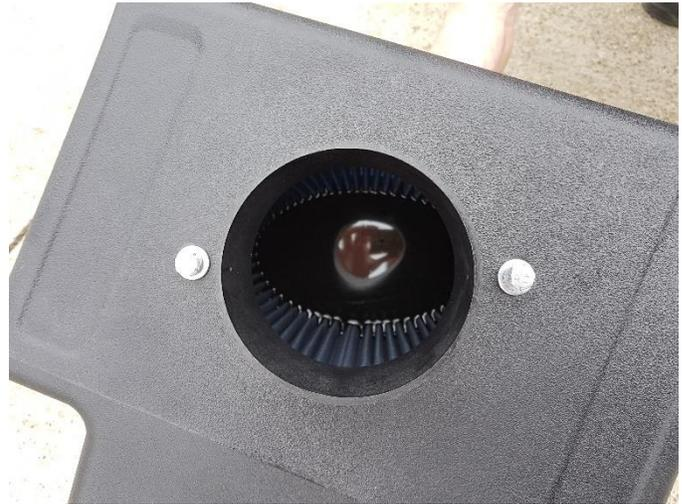
**7.** Secure adapter to airbox using a 10mm socket and ratchet.
