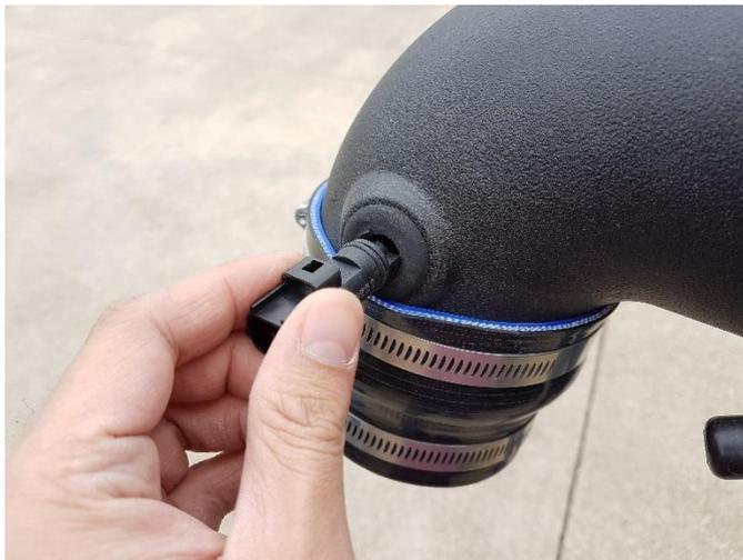
**1.** Carefully insert the stock air temperature sensor into the Corsa air duct. **NOTE:** The use of soapy water solution on the inside of the grommet might help to insert the sensor..
