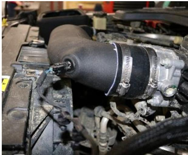
**12.** Connect ATS wiring harness onto sensor.
