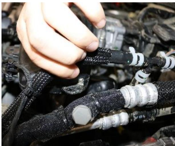
**3.** Using a trim removal tool, remove the clip securing the coolant hose to the factory air duct.
