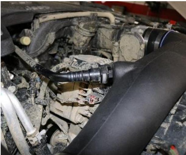
**11.** Connect factory breather hose to quick connect fitting in CORSA air duct.
