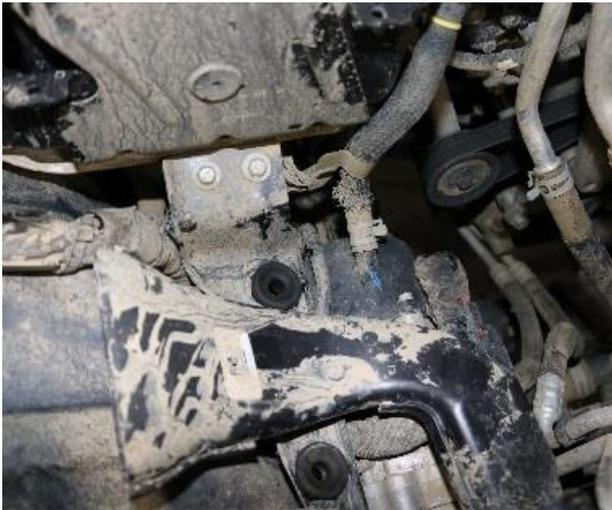
1. Locate the two factory grommets from removal step 9 and install them back into the factory location beneath the air box.
