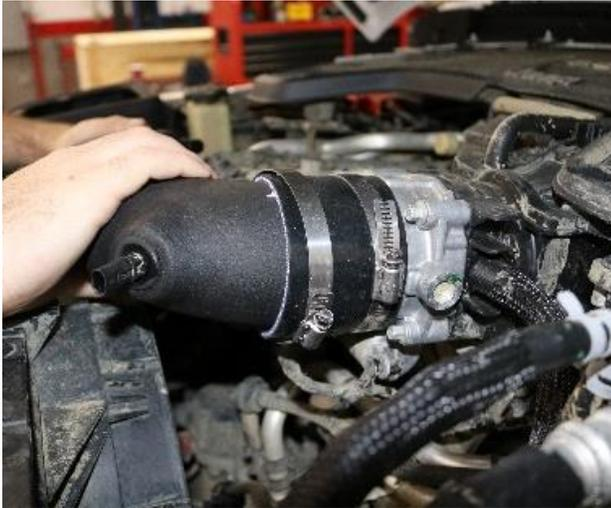
**9.** Install the straight sleeve onto the throttle body.
