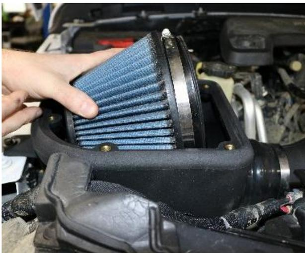
**13.** Locate either MaxFlow 5 Oiled Filter 5120 or PowerCore Filter 61513 and install into air box onto filter adapter.
