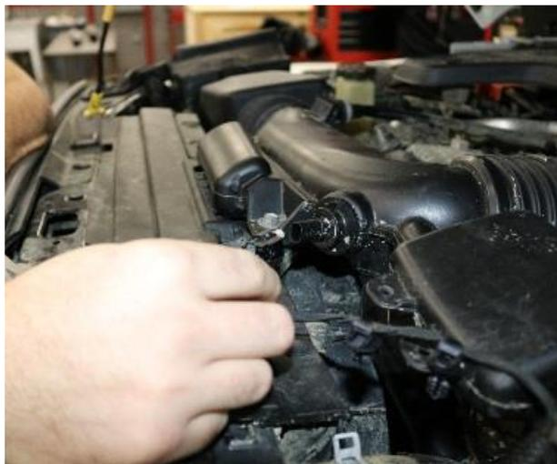
**1.** Unclip wiring harness for air temperature sensor.
