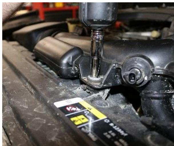
**4.** Remove the two bolts securing the factory air duct to the core support with a ratchet and 10mm socket.
