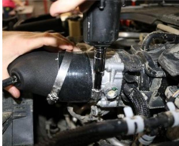
**10.** Adjust air duct as necessary and tighten all four clamps using a flathead screwdriver or ratchet and 8mm socket.
