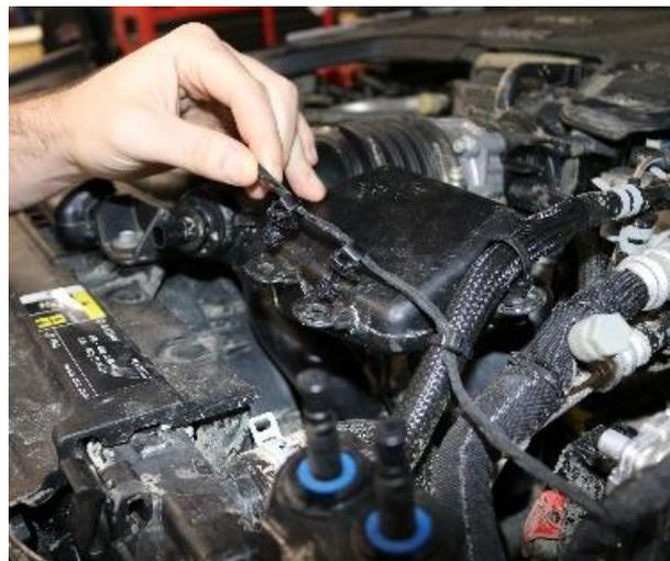
**2.** Using a trim removal tool, remove the two clips securing the ATS wiring harness to the factory air duct.
