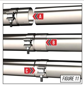
To accomplish the best tip fitment, align the 2.25" tip clamp to cover *only* the slot, as shown by **Arrow A** in **Figure 12**.
