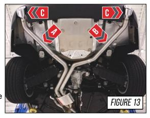
Once the exhaust tips are properly aligned, starting at the downpipe section moving towards the rear of the car, torque each Accu-Seal clamp to 40ft/lbs.
