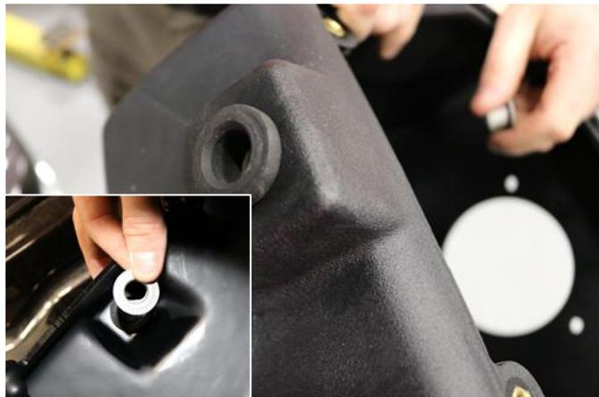
**1.** Locate CORSA air box and rubber grommet and metal bushing from removal step 9. Install grommet into air box the bushing into grommet from inside box.
