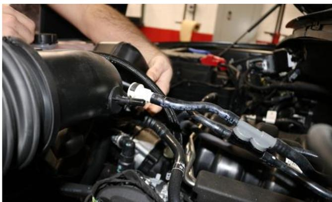
3. Disconnect both vent connections from rear of factory air duct.
