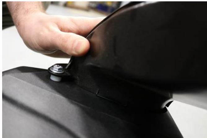
**2.** Locate the factory scoop from removal step 10, the 6mm x 25mm bolt, one .25" x .63" flat washer, the .25" x .75" flat washer, one .25" lock washer, the .25" spacer, and the 6mm nut. Attach air scoop to air box placing the spacer between the scoop tab and air box. Tighten hardware with 10mm wrenches.
