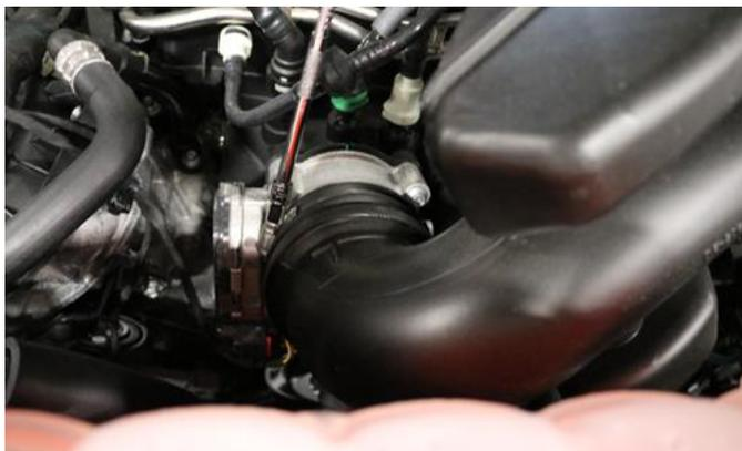
1. Loosen the clamp securing the factory air duct to the throttle body using a flathead screwdriver or ratchet and 7mm socket.
