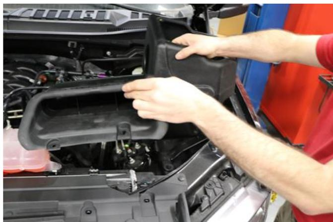
**3.** Install CORSA air box with scoop into the vehicle by inserting posts on bottom of CORSA air box into factory grommets.
