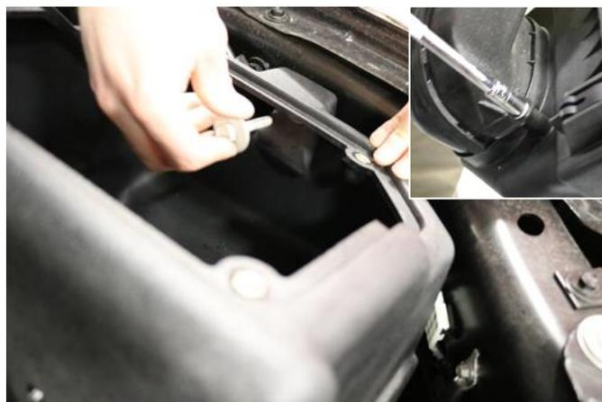
**4.** Locate the bolt from removal step 7 and attach the CORSA air box to the inner fender using a ratchet and 13mm socket.
