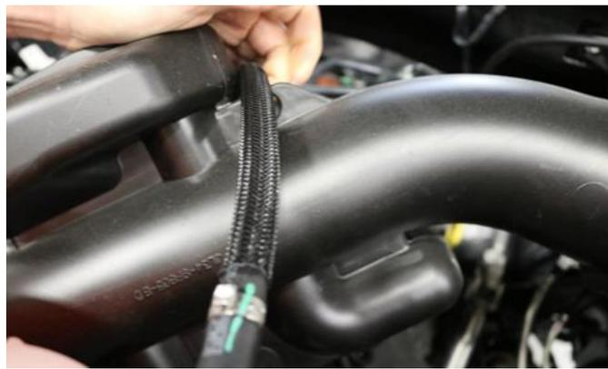
2. Pull the coolant hose from retaining feature on factory air duct.
