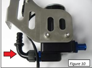
Mount the new pump using the same two studs as the factory pump. Apply blue Loctite to the factory studs and reuse the factory nuts to secure the pump.
