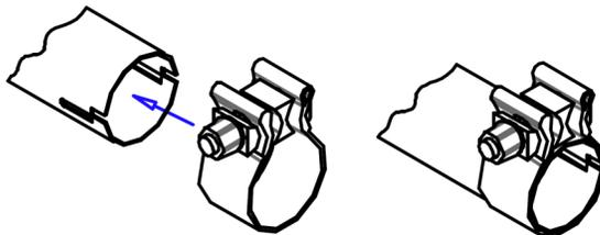
**WARNING:** Use extreme caution during installation. Torque all fasteners according to manufacturer's torque values and tightening sequence. **DO NOT** use air impact tools to tighten fasteners on Borla Performance Exhaust Systems. Use of such tools may result in bent flanges or gasket contact areas leading to exhaust leaks.
