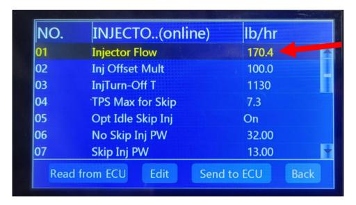
4. Scroll down the Injectors and VFI section until you find Injector Offset. Input the data into each section from the injector data sheet you opened from the website. This is continued further below.
