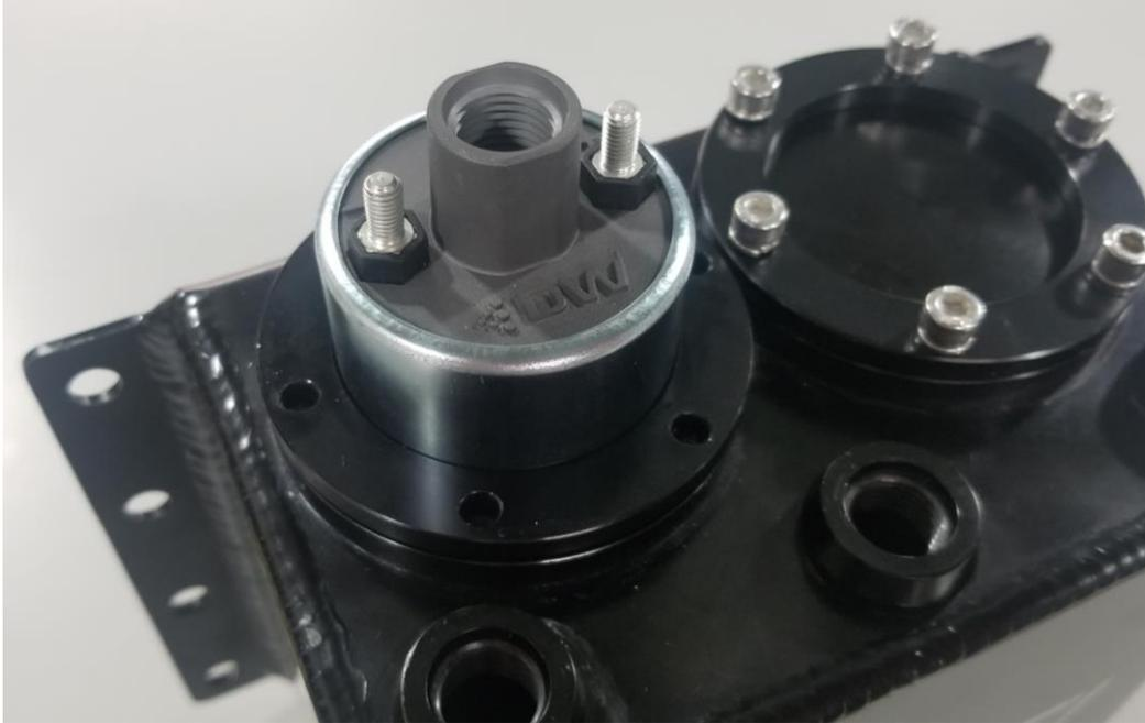
6 – Install Retaining ring on top of pump with the 6 retaining bolts and lock washers.
