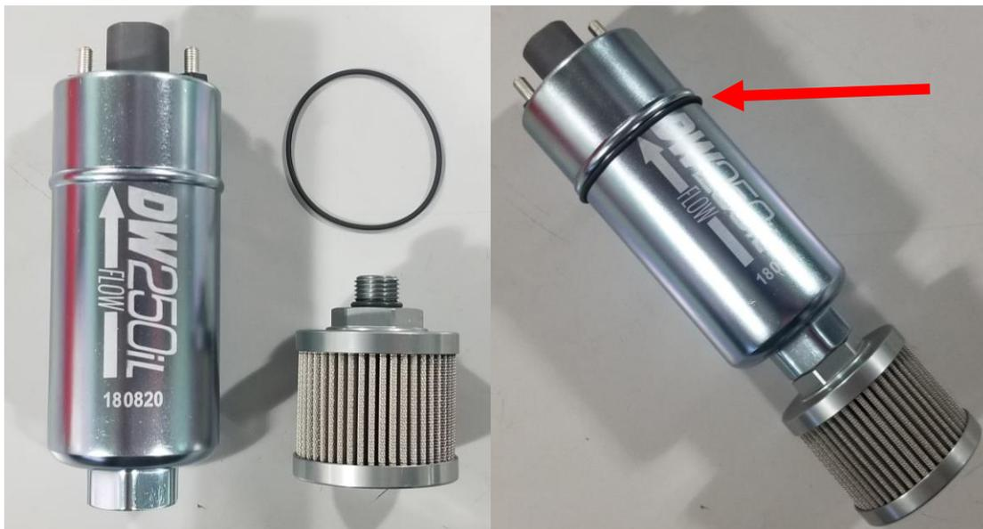
5 – Install Pump w/ filter. The o-ring on the bottom of the pump's retaining ridge should hold it in place. Make sure o-ring is not pinched or protruding from any side.
