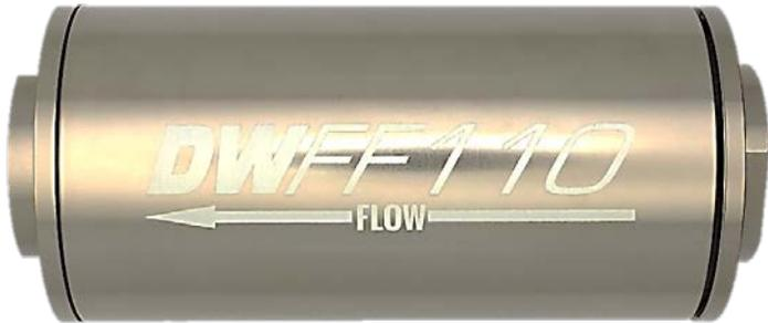
DW fuel filters are compatible with a wide range of fuels including pump gas, race gas, MTBE, ethanol, methanol, and diesel. DW recommends a maximum service interval of 12 months or 12,000 miles. Shorter service intervals are recommended with harsher conditions and corrosive fuels.
