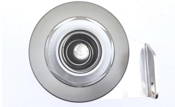
4 – The supplied mounting brackets are retained by the housings end caps. These can be orientated 4 different ways. There are 4 flats machined into the brackets and the housings, these can be rotated every 90-degrees to change the mounting angle. Make sure the brackets are sitting flush before fully tightening the end caps.
