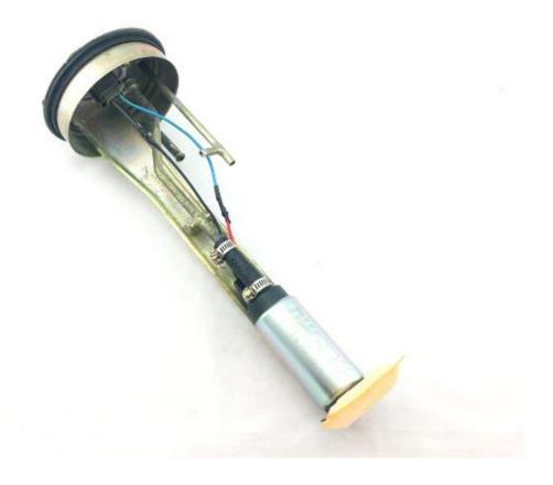
5 – reinstall the assembly into the fuel tank and attach a length of hose to the outlet of the pump assembly allowing it to drain into a fuel safe container and prime the fuel pump assembly
