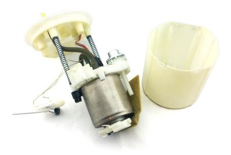
2 – plastic hoses have to be cut for removal and cannot be reused. Take note of wire routing and connections
