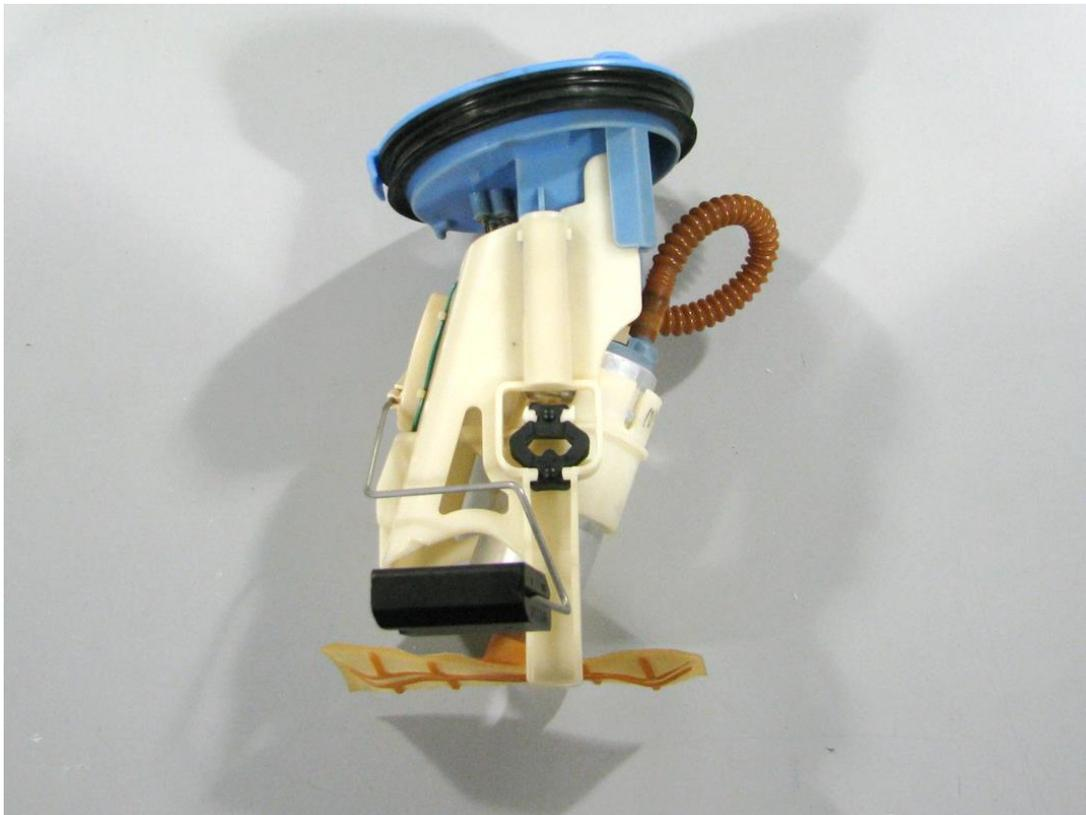
1 – remove the OE fuel pump from the assembly by cutting the electrical connector leads (leaving enough room to wire-in the new connector) and cutting the OE plastic tubing from the assembly. Use caution to not gouge the assembly inlet
