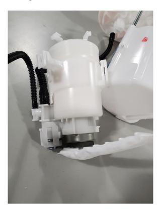
8 – Fold the flap of the filter sock up against the filter center section and install the whole assembly back into the bucket, re-latch the locking tabs, by pushing down on the center section firmly until they click into place. **Note**: For the Accord module re-attach the top hat to the bucket by compressing the springs and re-inserting the e-clip.
