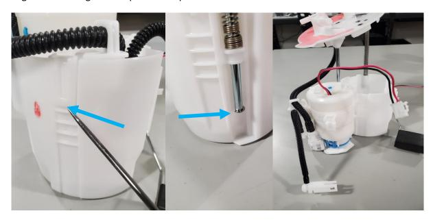
4 – Remove the factory fuel pump by unlatching the filter sock from the bottom of the filter center assembly. The pump may be held in place by the O-rings, you can push on the pump from the top connector side to remove it. Be sure to remove the O-ring from the center filter section if it remains in place and not on the pump.
