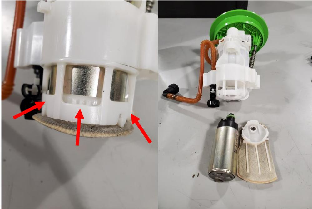
6 – Remove the spacing cage the OEM pump slid into. There are 4 locking tabs around the diameter of the module. The cage will not be reused if damage is done during removal.
