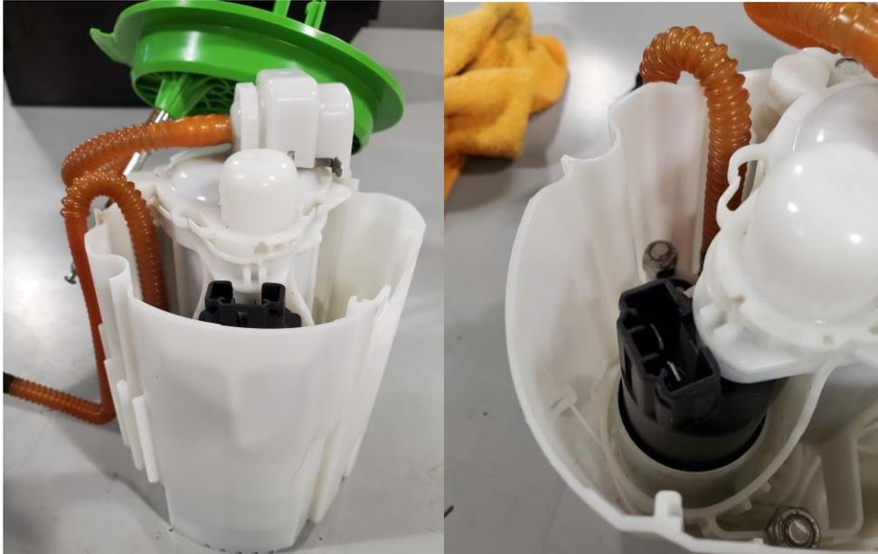
10 – Reinstall the venturi line on the side of the bucket and install the supplied fuel pump connector onto the DW pump. You can now either use the supplied fuel safe heat shrink butt connectors to crimp the factory wiring to the DW wiring, or you can solder the supplied connector to the factory terminals. Combine the factory brown static ground wire with the black DW wire when soldering or crimping.
