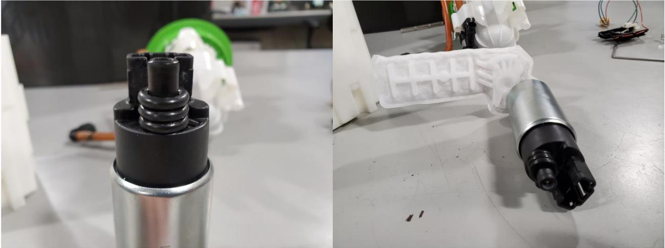
8 – Install the pump into the center section, seating two of the O-rings all the way into the module, the 3<sup>rd</sup> O-ring acts as a spacer to prevent the other two from pushing down with fuel pressure.
