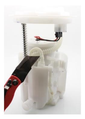
2 – disconnect the electrical connector for the pump from the hat of the assembly; it may also be easier to work with the assembly if the fuel level sensor is disconnected as shown in the pictures
