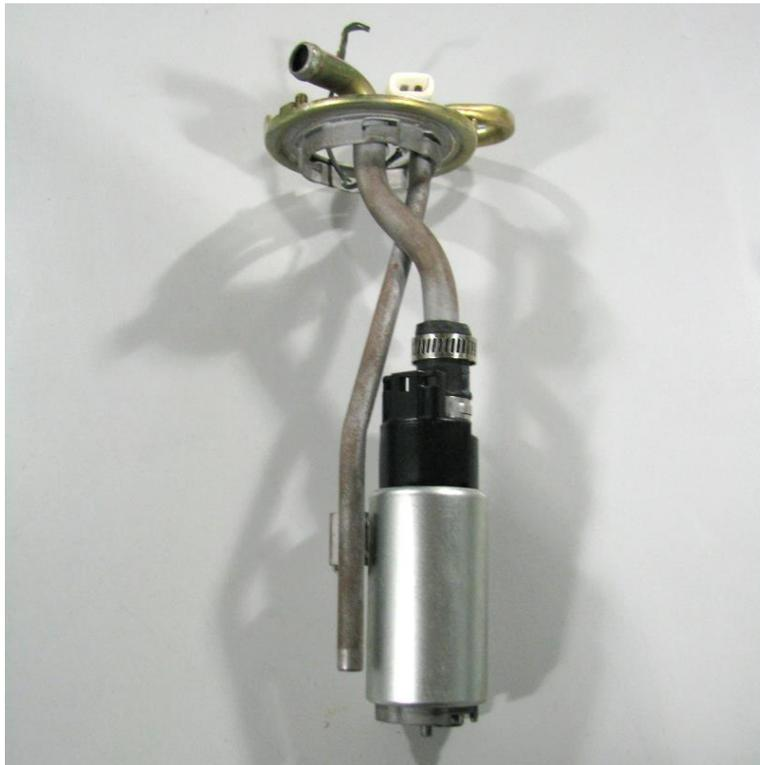
3 – wire-in the supplied electrical connector. Secure the DW65c/300c to the assembly with the supplied zip-tie and install the pump pre-filter (fuel sock) onto the DW65c/300c
