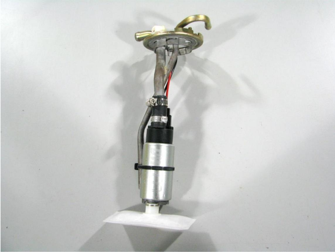
4 – reinstall the assembly into the fuel tank and attach a length of hose to the outlet of the pump assembly allowing it to drain into a fuel safe container and prime the fuel pump assembly
