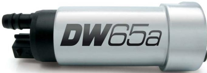
The DW65a in-tank fuel pump with install kit was specifically designed for the Holden Commodore Gen III 97-06 5.7/6.0 V8 but also fits other popular applications (see application guide). The DW65a flows 265lph at 40psi and features a quiet and reliable turbine impeller which is compatible with pulse width modulated pump drivers. The pump also features an encapsulated armature for compatability with ethanol based fuels. All DW fuel pumps are backed by a 3-yr no fault warranty.
