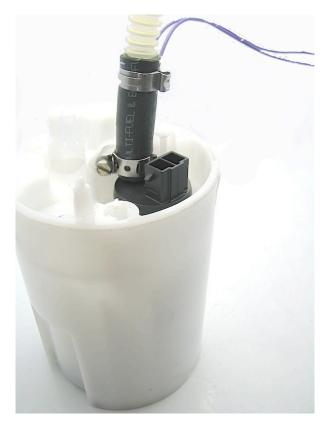
9 – connect the convoluted tubing to the upper assembly and secure with the hose clamp, then reinstall the top assembly to the lower assembly
