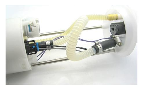
10 – reinstall the assembly into the fuel tank, then crank the engine for a period of time long enough to prime the pump assembly and evacuate the air introduced during the pump installation process
