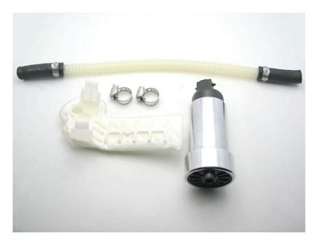
7 – install the DW65a into the center assembly by clicking the tabs on the fuel sock into place and then reinstall the center assembly into the lower assembly
