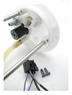
2 – carefully remove the tube connecting the fuel pump the fuel pump assembly, by cutting it with a sharp knife
