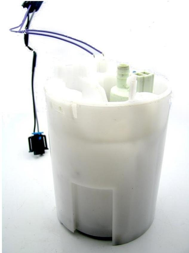
4 – remove the center assembly from the lower assembly by depressing the 3 tabs (green) and pull up on the center assembly, away from the lower assembly
