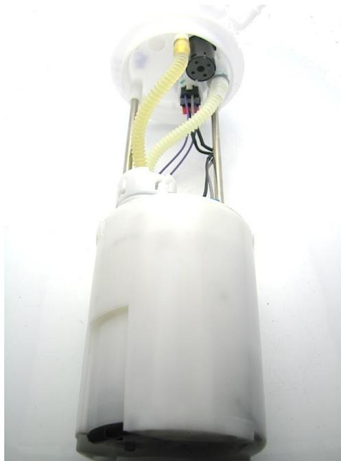
1 – disconnect the main connector for the fuel level sender and fuel pump electrical connector
