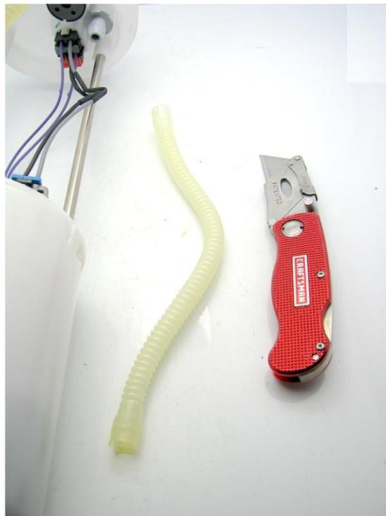
3 – disconnect the fuel pressure regulator (green) by prying it up and out of the pump assembly, then pull the top of the assembly from the bottom using a similar motion as a slide hammer
