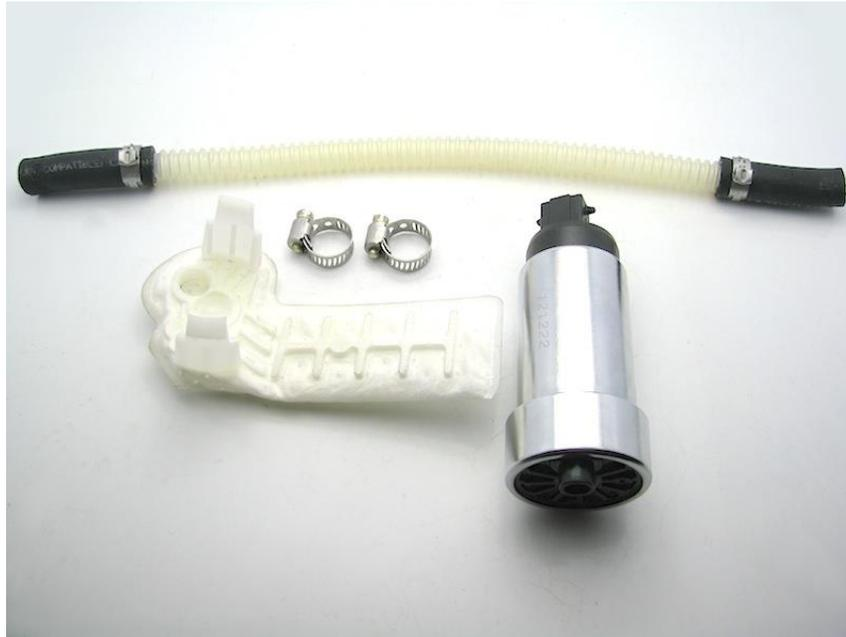
7 – install the DW65a into the center assembly by clicking the tabs on the fuel sock into place and then reinstall the center assembly into the lower assembly
