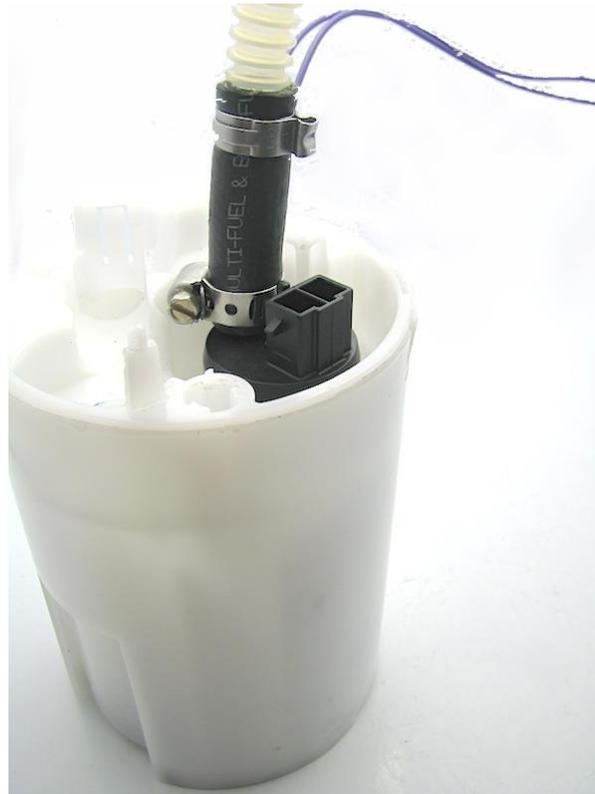
9 – connect the convoluted tubing to the upper assembly and secure with the hose clamp, then reinstall the top assembly to the lower assembly
