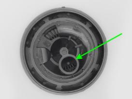
7 – install the new fuel hose supplied on the 65v and then install to the top of the assembly
