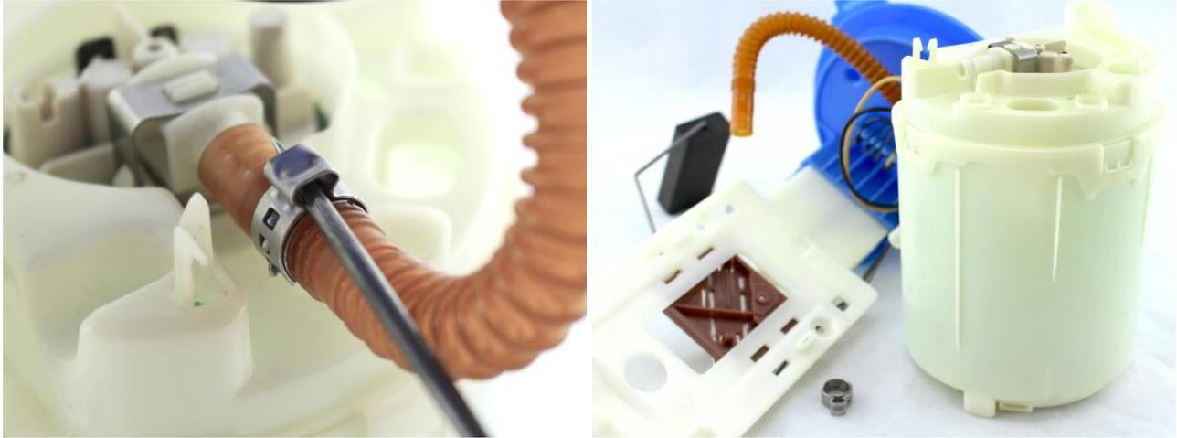
4 – Removed the bucket cap by lifting the four tabs around the top (circled in green), the pump will come out with the cap with a gentle pull
