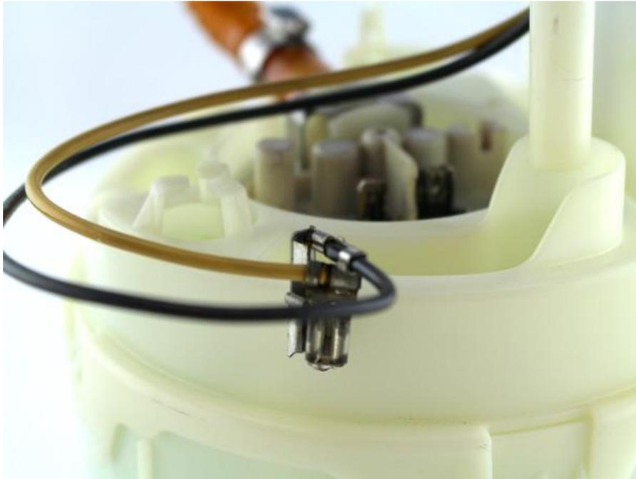
2 – Remove the screws that attach the top of the assembly to the bucket, these can be either a 7mm hex or T20 Torx
