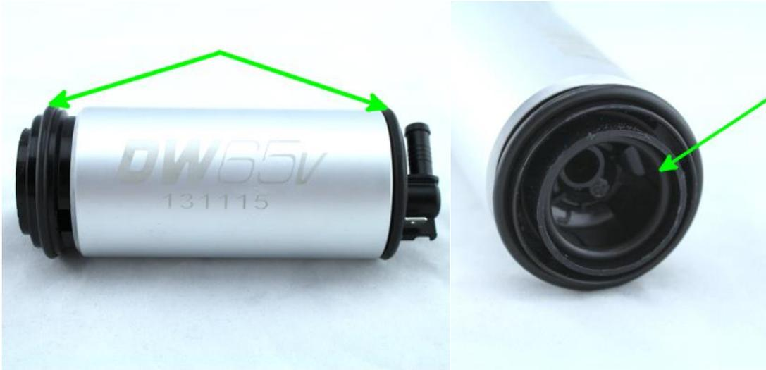
5a – The proper location for the larger lower O-ring is below the lip and leaves the rectangular port on the cap exposed (circled in green)
