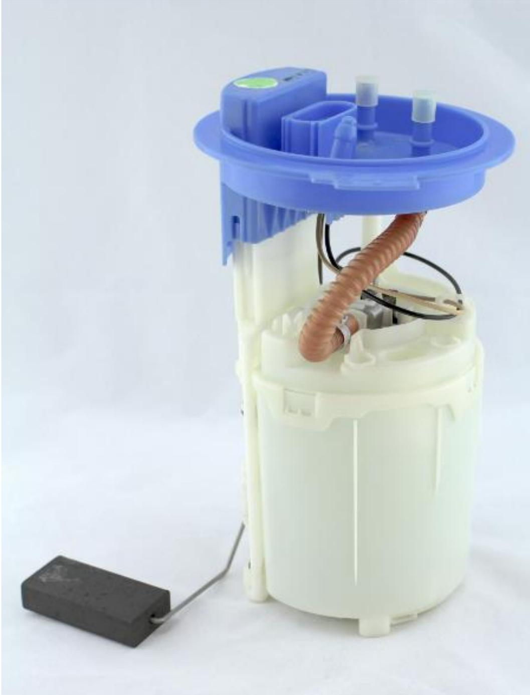
1 – Unplug the electrical connectors, both connectors have tabs that need to be pushed in as the connector is pulled up
