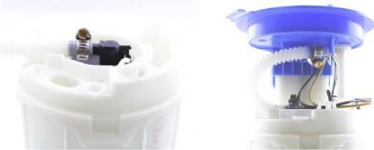
8 – Reinstall the top and connect the wires to the pump
