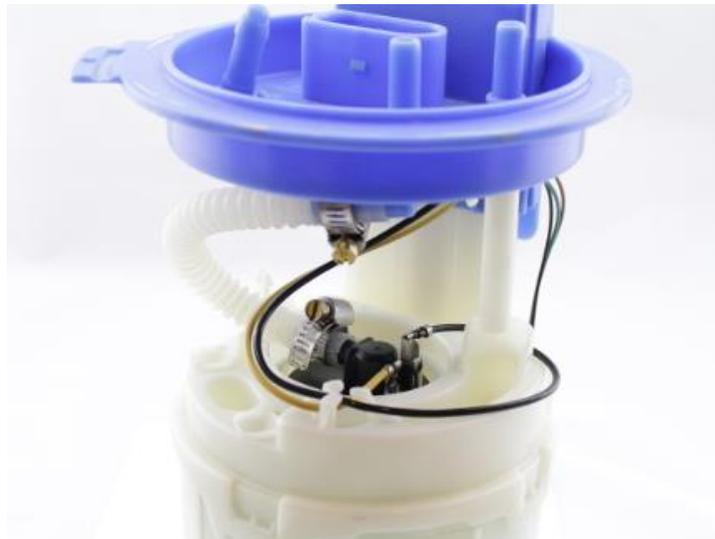
9 – AWD models will connect the factory venturi/siphon tube to the small outlet barb on the top of the fuel pump.
