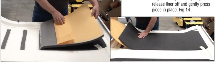
FIG. 14 Peel back a small section of release liner start to adhere the piece to the top. Continue to pull the relase liner off and gently press piece in place
