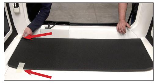
8.) Lay correct piece in removable top. Once again use painters tape to temporarily hold pice in place. Fig 9
