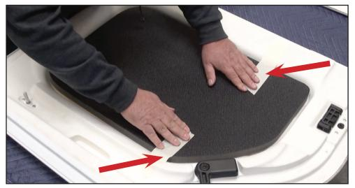
5.) Lay correct piece in freedom top and get properly alligned. Use painters tape to temprarily hold piece in position. Fig. 5
