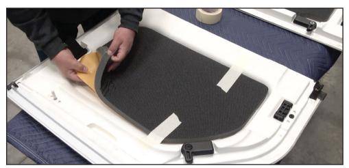
6.) Peel off backing at one end of the freedom top piece and adhere to the top. Use slight pressure to stick it down. This will hold the piece in place. Fig 6
