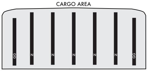
3.) Test fit the filler strips into the ribs of corresponding length before peeling the release liner on the strips. Refer to proper diagram on page 2 for proper placement of filler strips.
