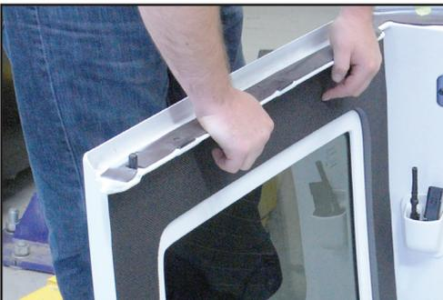
2.) Test fit to determine the correct placement for each side.
