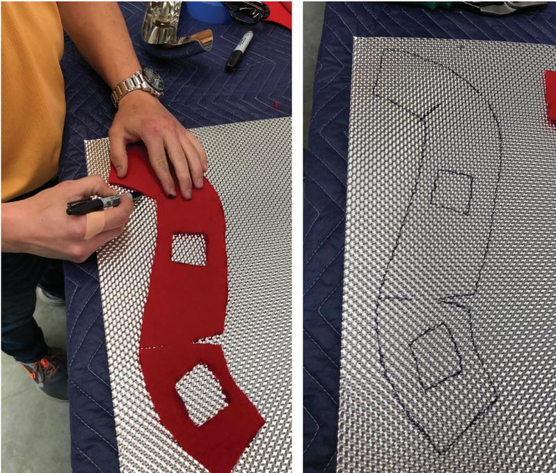
13. You will need to transfer the pattern to the aluminum. Lay the pattern on the aluminum and trace with a marker. Make the line slightly smaller than the felt pattern, just the width of the marker line will do. (Fig 12)
