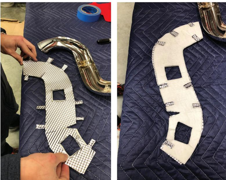
17. Lay the insulation on top of the aluminum, make sure you have the correct orientation to fit the shield. Bend over the tabs to hold the insulation in place. (FIG 16)
