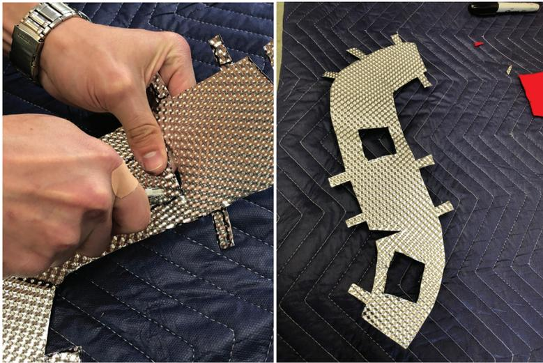
15. Use a utility knife to cut out the center holes for the clamp standoffs. (FIG 14)
