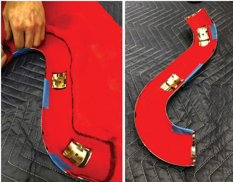
9. Trace a cut out line on the other side of the felt. Cut along the line using scissors (Fig 8)
