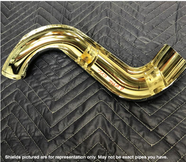
**STEP 1.** Allow the motorcycle to cool before performing any work. Remove your heat shields following the factory manual. Most are held in place with worn gear style clamps. Once the shields are removed, mark the direction the clamps are installed, then remove the clamps from the shield.
