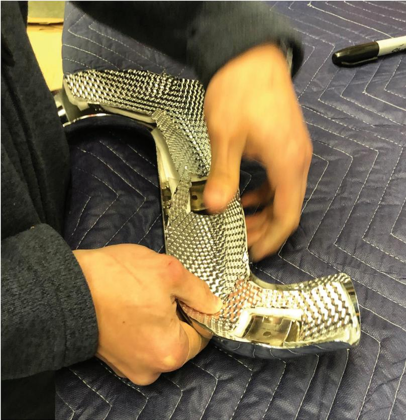
18. Lay the heat shield liner into your pipe shield and press into place. This will take a little time to get the fit correct. You may have to trim some material once its in place. (fig 4245 and 4246)
