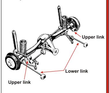
NOTE: All 4 control arms (2 upper 2 lower) use the same bushing for all 8 positions. Factory rubber bushings are not bonded.
