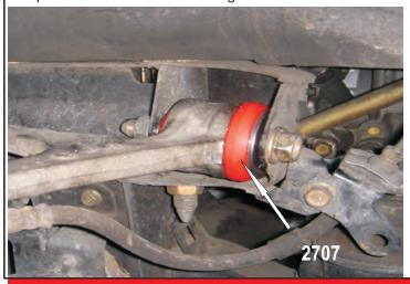
STEP 2: After the stock sleeve has been removed, use a hacksaw to cut tabs on both sides of the stock outer shell. (Note: Upper control arm shown below 2707 2 PLACES)
