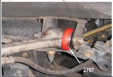
STEP 2: After the stock sleeve has been removed, use a hacksaw to cut tabs on both sides of the stock outer shell. (Note: Upper control arm shown below 2707 2 PLACES)
