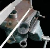
STEP 3: Using a cold chisel, bend back the tabs to make room for a piece of tubing to fit
