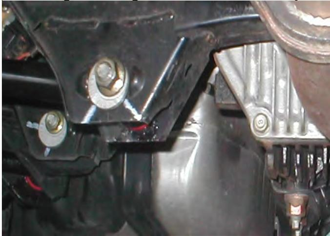
Typical bushing setup for all lateral and trailing links pictured below. After stock bushing and sleeve has been removed, clean and lubricate the inner surface prior to installing the new bushing set. Grease the outer flange of the bushing prior to installing the link back into the frame.
