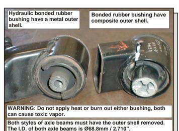
Securely hold the axle beam in a vice and use a bushing driver to drive out the O.E. Bushing.
