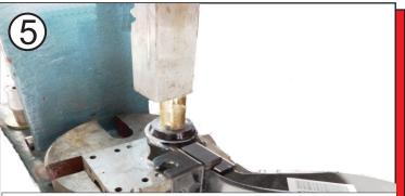
Grease the I.D. of track arm, I.D. & O.D. of bushing 03P03605 and O.D. of sleeve 15P1071639 (inner position) and sleeve 15.10.419.39 (outer position). Press in bushing 03P03605 first, then press in the inner metal sleeves 15P1071539 and 15.10.419.39.
