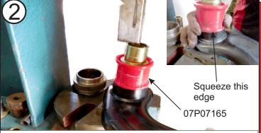
Grease the I.D. of trailing arm, I.D. & O.D. of bushing 07P07165 and O.D. of sleeve 15P1071539. Press in bushing 07P07165 first (squeeze the leading edge of bushing to help get it started into the eye) then press in the inner metal sleeve 15P1071539.
