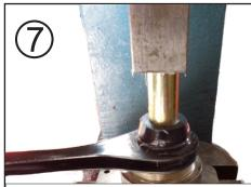
Grease the I.D. of tie rod, I.D. & O.D. of bushing 03P03604 and O.D. of sleeve 15.10.472.39 (inner position) and 03P03603 and sleeve 15.10.419.39 (outer position). Press in bushing 03P03604 and 03P03603 first, then press in the inner metal sleeve 15P1071539 and 15.10.419.39, respectively.
