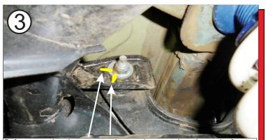
Before removing the upper track arm, place matchmarks on the front and rear of the adjusting cam bolts. You will need to use these matchmarks to reinstall the track arm back in the same position after the new polyurethane bushings are installed.
