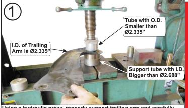
Using a hydraulic press, properly support trailing arm and carefully press out the rubber bushing with bonded outer metal casing.
