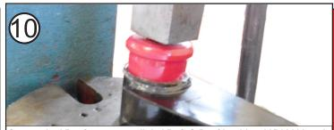
Grease the I.D. of transverse link, I.D. & O.D. of bushing 03P03602 and O.D. of sleeve 15.10.472.39. Press in bushing 03P03602 first, then press in the inner metal sleeve 15.10.472.39.
