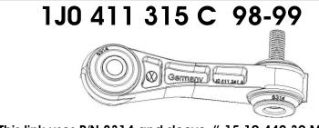
This link uses P/N 8314 and sleeve # 15.10.442.39.Must reuse O.E. shoulder bolt at bar end.
