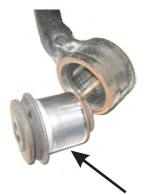
Factory bushing metal shell must be pressed out of upper control arm for Energy Suspension polyurethane bushings to fit properly.
