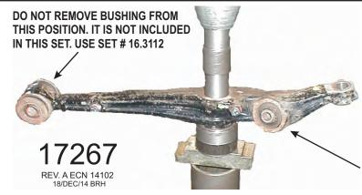
A hydraulic press was used to remove the original bushing, including the outer metal casing the rubber is bonded to. The inside diameter of the control arm is Ø 36mm (1.417"). Go about .050" smaller when pressing out the bushing. Grease all sides of the bushing that contact metal. Press in the Energy Suspension bushing 2357. Grease sleeve 15.10.88.39 and press into the bushing.
