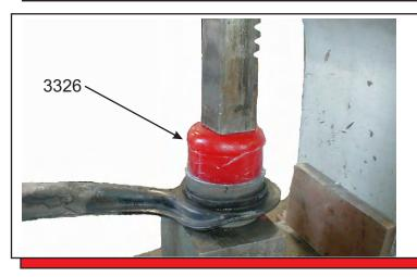
Let metal shell cool before cleaning inside. Remove any burrs and sharp edges before applying grease. Clean the hole/barrel in the control arm that you just removed the bushing from. Lubricate the inside of the hole/barrel. Grease all sides of the bushing that contact metal. Press in the Energy Suspension bushing 3326. Grease sleeve 15.10.357.39 and press into the bushing.
